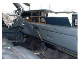
Figure 13 Angular view of the instrument panel showing the front right air bag module cover
