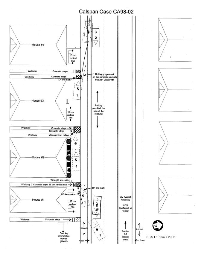
Figure 7. Scaled scene schematic
