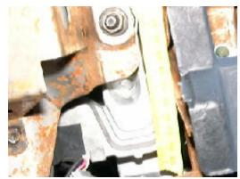
Figure 10 View of the shear capsule displacement
