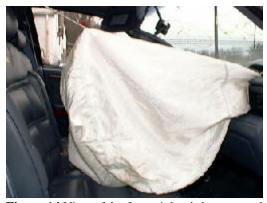
Figure 14 View of the front right air bag manual expanded to illustrate bag excursion
