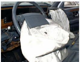
**Figure 11** View of the front left air bag module cover flap and air bag
