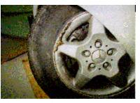
Figure 8. Asphalt embedded into the left front wheel which tripped the ML 320.
