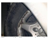
Figure 12. Close-up view of the embedded asphalt into the left front alloy wheel.
