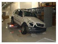
Figure 10. Rollover damage to the right side area of the vehicle.
