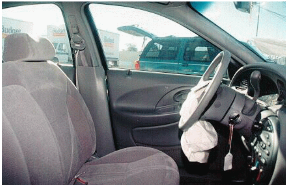
Figure 13: Case vehicle's driver seating area; Note: three-point, lap-and-shoulder, safety belt system (case photo #37)
