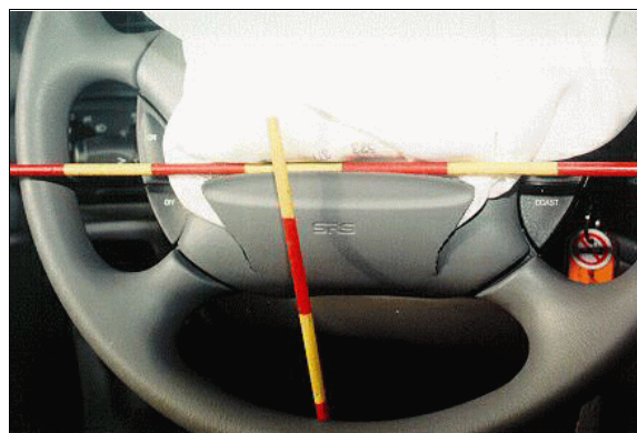
Figure 7: Case vehicle driver air bag module's lower cover flap (case photo #36)
