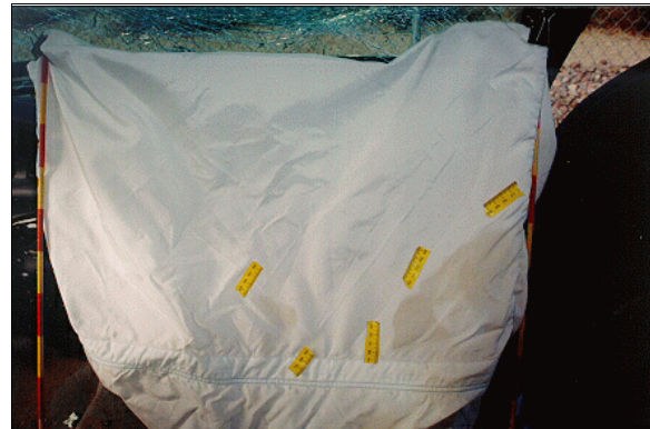
Figure 10: Case vehicle's front right passenger air bag; Note: soda stain at lower left and large coffee stain at lower right (case photo #51)
