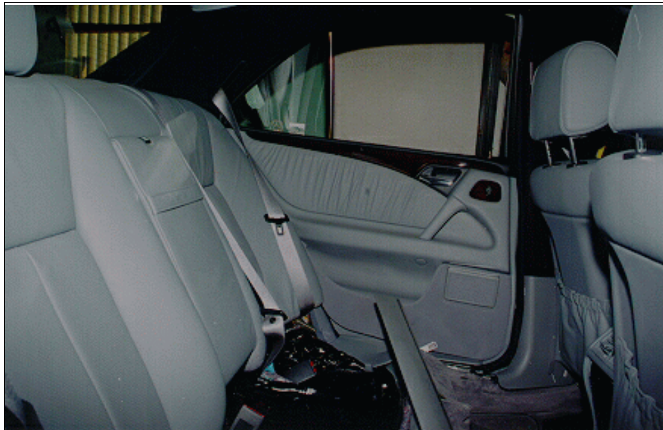
Figure 7: Case vehicle's back seat showing intruded left rear door and removed left rear seat cushion (case photo #36)
