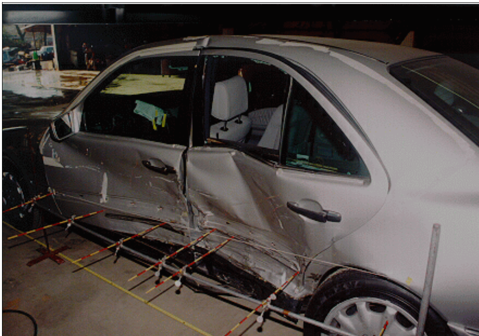
Figure 3: Case vehicle's damaged left side, looking forward (case photo #14)
