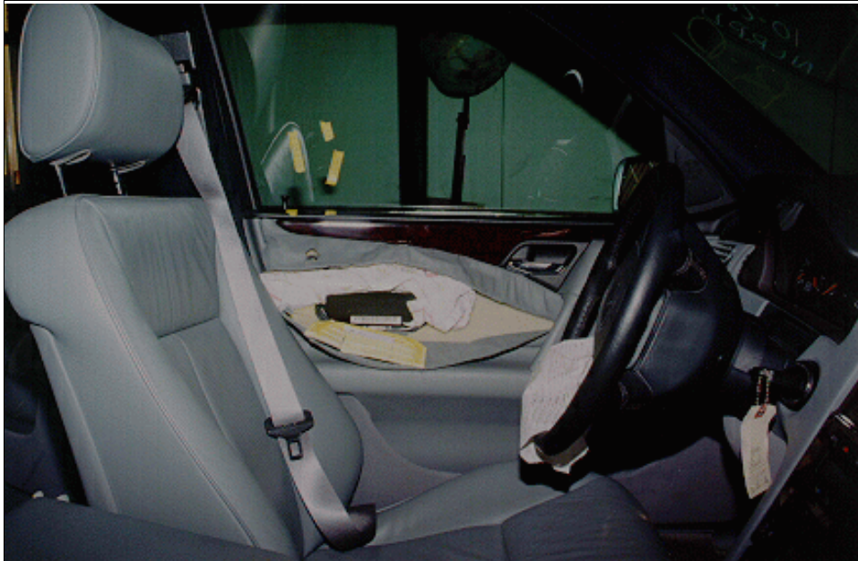
Figure 4: Case vehicle's driver seating area and left side air bag module (case photo #22)
