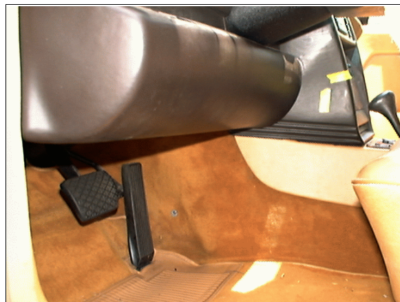
Figure 11: Case vehicle's driver knee bolster and left side of center instrument panel showing no contact evidence on knee bolster and driver's right knee contact to instrument panel (case photo #32)
