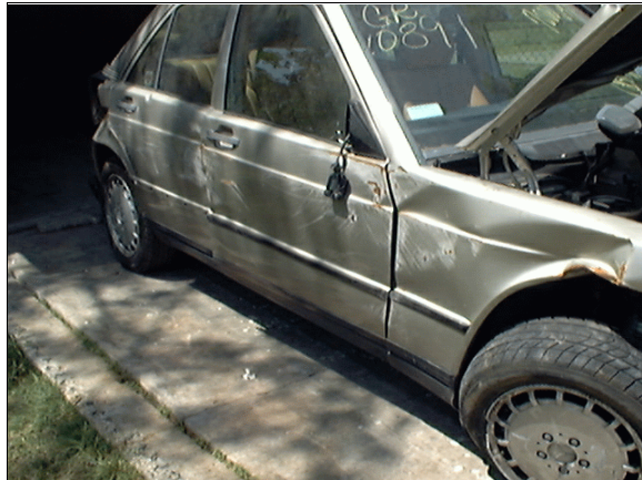
Figure 7: Case vehicle’s right side damage from slapping impact with median guardrail (case photo #24)
