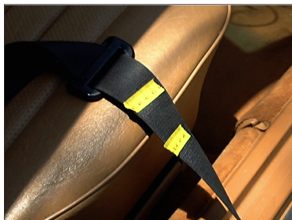
Figure 16: Case vehicle's front right safety belt showing heat abrasion mark on belt's webbing (case photo #42)
