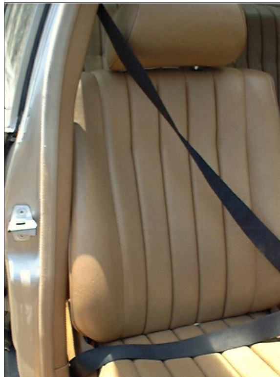
Figure 15: Case vehicle's front right safety belt system showing belt fully extend and not retractable because pretensioner had actuated accompanying deployment of driver's air bag (case photo #43)
