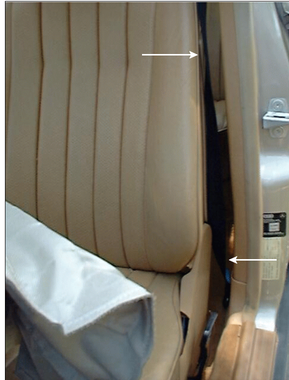
Figure 14: Case vehicle’s driver safety belt system shown along “B”-pillar with belt webbing free to reel in and out; Note: emergency tension retractor did not actuated when air bag deployed because safety belt was not buckled (case photo #44)
