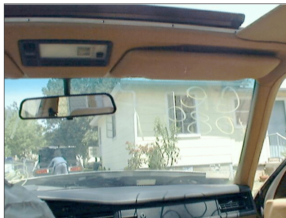
Figure 18: Case vehicle's center and front right greenhouse areas showing no obvious occupant contact evidence (case photo #31)
