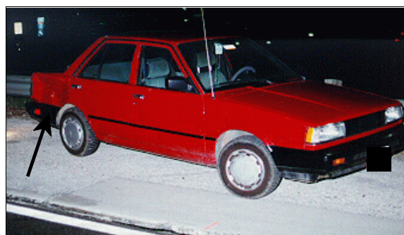
Figure 3: On-scene photo looking south-southeast at Nissan's final rest position on south shoulder; Note: sideswipe damage to right quarter panel from impact with case vehicle's left front fender (case photo #13)
