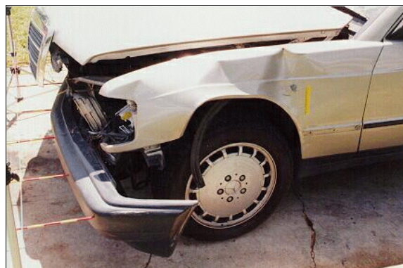
Figure 2: Damage to case vehicle's left fender from initial sideswipe impact with Nissan's right quarter panel (case photo #18)
