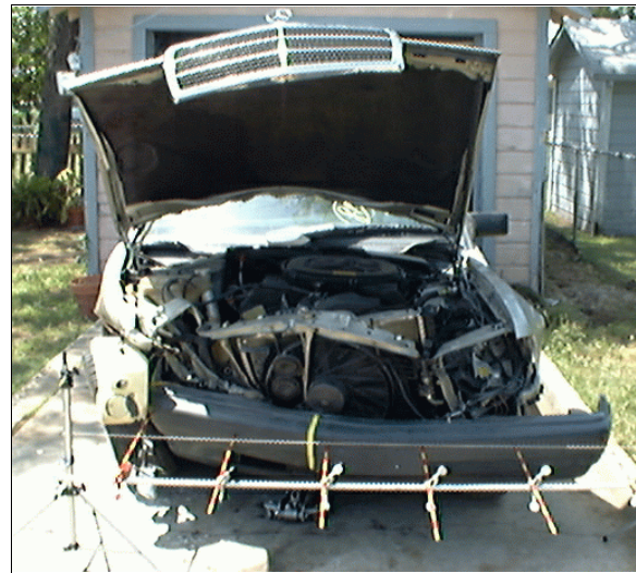
Figure 6: Case vehicle's frontal damage with contour gauge present; Note: yellow tape marks leftward end of direct damage and leftward shift of front bumper (case photo #15)
