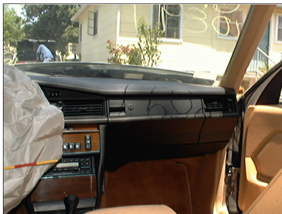
Figure 19: Case vehicle’s front right instrument panel and windshield’s glazing showing no obvious occupant contact evidence (case photo #40)
