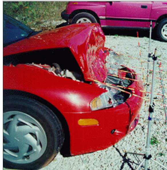
Figure 4: Case vehicle's front underride damage viewed from right along front reference line (case photo #22)
