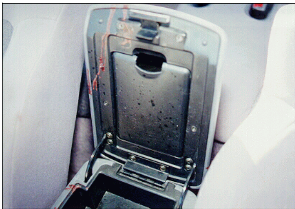
Figure 11: Inside surface of case vehicle's console storage area cover showing bloodstains, indicating that cover was raised at time of crash (case photo #44)
