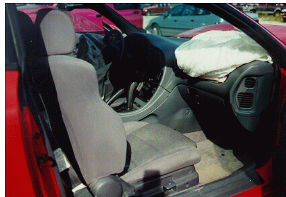
Figure 6: Case vehicle's front right seating area showing deployed front right passenger air bag and center console with floor-mounted, transmission selector lever (case photo #31)
