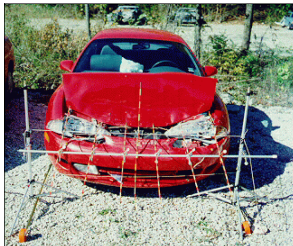
Figure 3: Underride damage to case vehicle's front with contour gauge showing above bumper damage (case photo #10)
