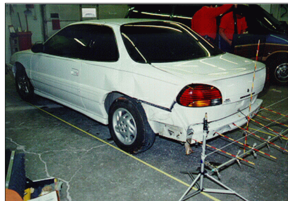
Figure 16: Pontiac's damaged back viewed from left of back; Note: induced damage to left quarter panel (case photo #64)
