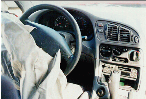
Figure 7: Case vehicle’s front seating area showing deployed driver air bag, center instrument panel, and automatic transmission selector lever (case photo #28)
