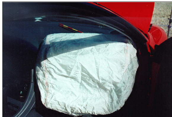
Figure 14: Case vehicle's deployed front right passenger air bag; Note: no visible contact evidence was found on this air bag (case photo #49)
