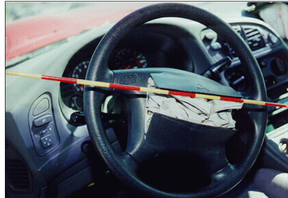
Figure 8: Case vehicle’s steering wheel showing driver air bag module’s top and bottom cover flaps and refolded air bag (case photo #32)
