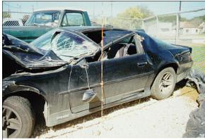
**Figure 6:** Direct contact to Chevrolet's hood and left roof rail, "A"- pillar, and upper "B"- pillar, viewed from front of left (case photo #65)
