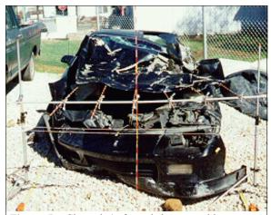
Figure 5: Chevrolet's frontal damage with contour gauge present and positioned above bumper; Note: contact to top of hood (case photo #60)
