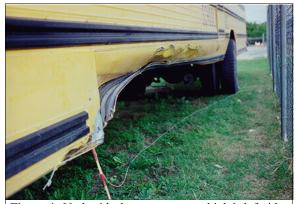
Figure 4: Underride damage to case vehicle's left side (case photo #19)
