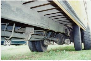
**Figure 9:** Contacts to case vehicle's left frame rail and drive train; Note: the positioning of the left rear tandem wheels (case photo #20)
