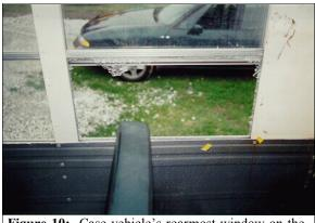
Figure 10: Case vehicle's rearmost window on the right side; Note: disintegrated window glazing and blood stains (yellow tape) on the interior side panel (case photo #56)
