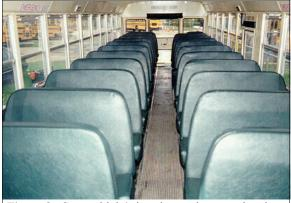
Figure 8: Case vehicle's interior seating area showing 65 passenger seating positions (case photo #45)
