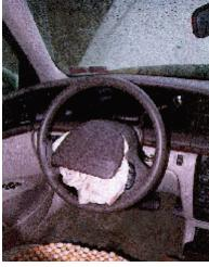
Figure 7. Vertically oriented abrasion pattern on the lower third of the upper module cover flap.
