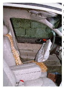
Figure 4. Profile view of the horizontal distance between the seat back support and the driver air bag module as documented by the officer.
