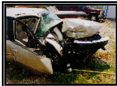
Figure 5. Impact damage to the front right of the Chevrolet Malibu.
