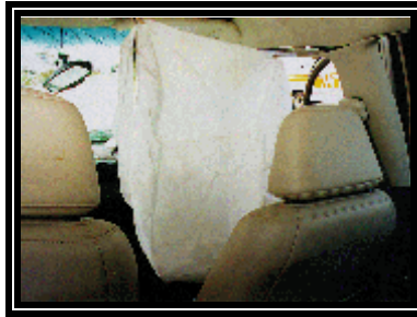
Figure 12. Trajectory of the child passenger into the deployed front right air bag.
