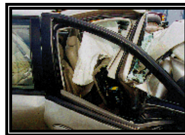
Figure 13. Intrusion of the right instrument panel into the front right passenger compartment.
