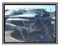
Figure 5. Left side damage to the 1995 Buick Century.
