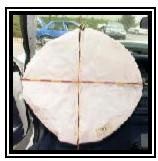
Figure 6. 1999 Ford Crown Victoria redesigned driver air bag.
