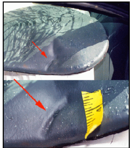
Figure 17. Fiber transfers, passenger side module cover
