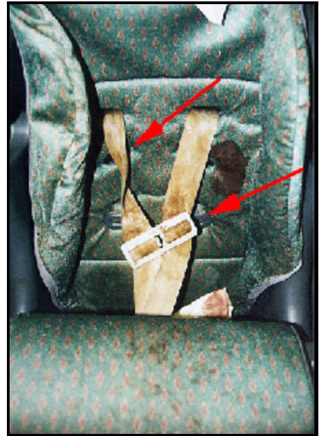
Figure 12. Child safety seat—chest clip and twisted harness
