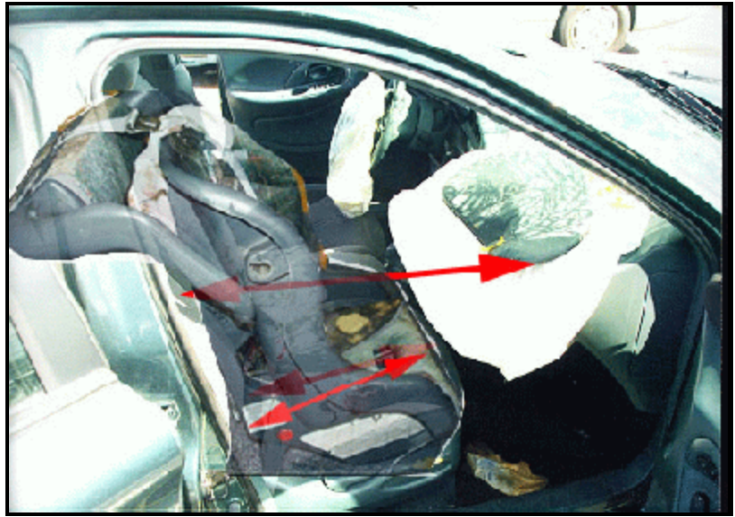
Figure 14. Front right seat with scaled image of child seat superimposed onto seat image.
