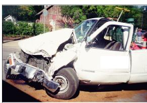
Figure 7: Chevrolet pickup's frontal damage viewed from left; Note: position of left front tire and induced damage to the left "A"-pillar (case photo #16)
