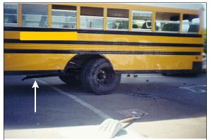
**Figure 4:** Damage to case vehicle's left rear wheel well and axle: Note: rearward displacement of left rear dual tires and disconnected drive shaft (case photo #10)
