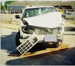
**Figure 6:** Chevrolet pickup's damaged front; Note: primary damage to front left corner and leftward shift of hood and right fender (case photo #15)
