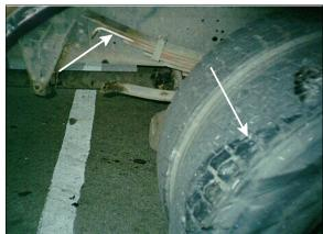
Figure 5: Forward end of case vehicle's broken left rear leaf springs; Note: Chevrolet pickup's contact marks on top leaf spring and on outside left rear dual tire (case photo #12)
