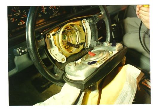
Air Bag Module Removed From Steering Wheel
