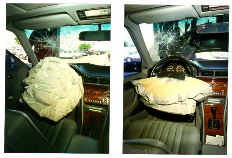
Overall Views Of The Driver's Seated Area, Related Contact Points, And Deployed Air Bag
