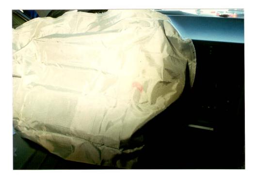
Lipstick Transfers On The Deployed Driver's Side Air Bag
