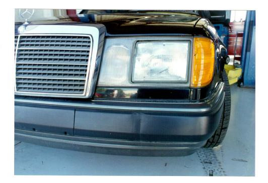
Direct Contact Damage On The Front Left Bumper Facia
