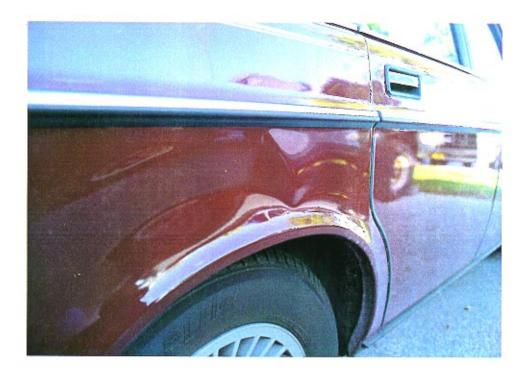
Remote Buckling To The Right Rear Quarter Panel Directly Over the Axle Position
