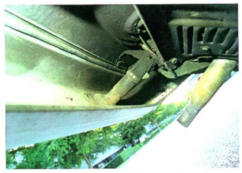
Compression/Stroke Of The Left Rear Bumper Energy Absorbing Unit
