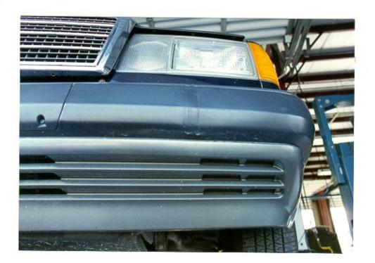
View Looking Upward At The Bumper Facia Deformation
