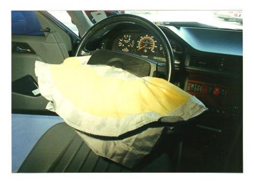
Closed Venting Panel On Upper Portion Of Air Bag
