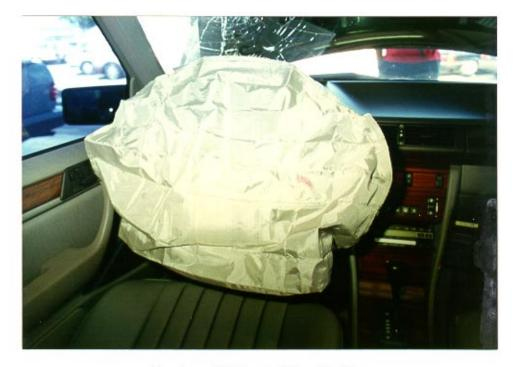
Deployed Driver's Side Air Bag
