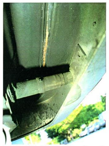
Compression/Stroke Of The Right Rear Bumper Energy Absorbing Unit
