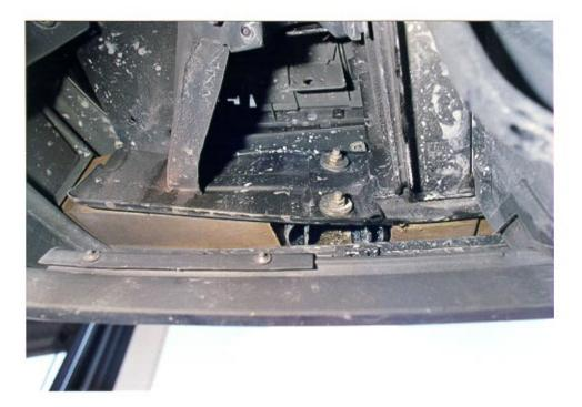
Undercarriage View Of The Backer Panel At The Left Front Corner (Arrows Indicate Deformation)
