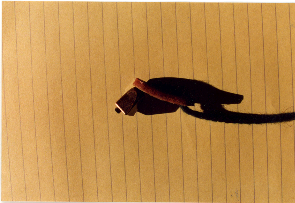
10. Plastic tab and leather slack adjuster which snagged in handrail/stairwell juncture.
