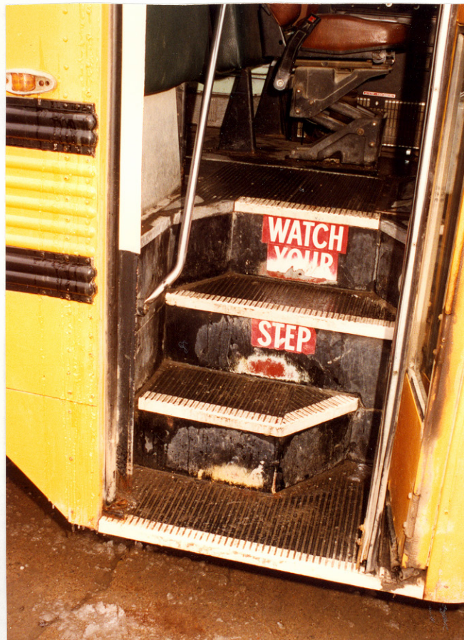
4. Interior view of the stairwell and post-accident modified handrail.
