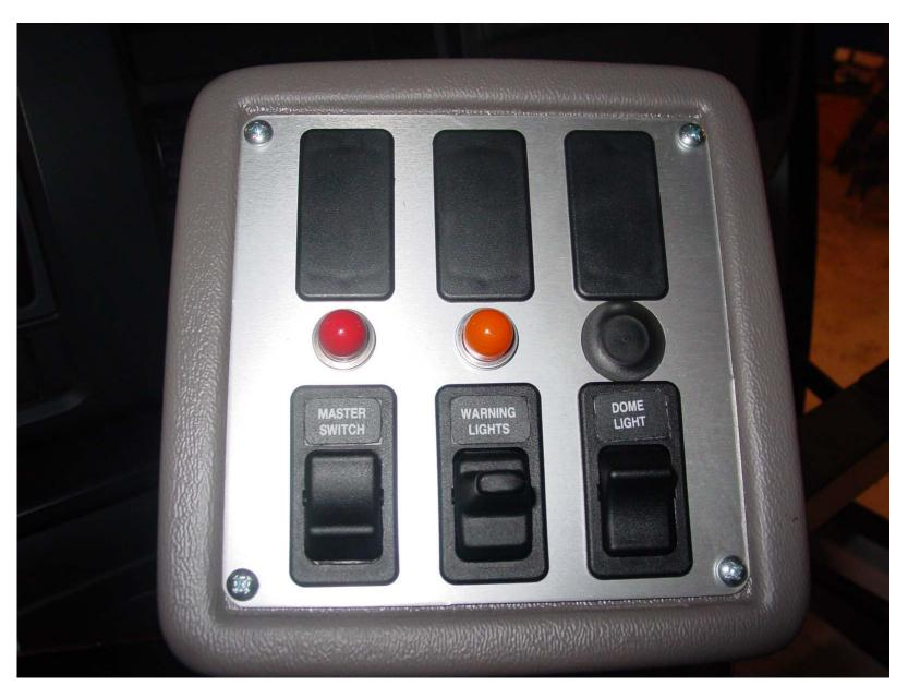
Close Up View of the Switches That Allow Extension of the Stop Signal Arm(s)
