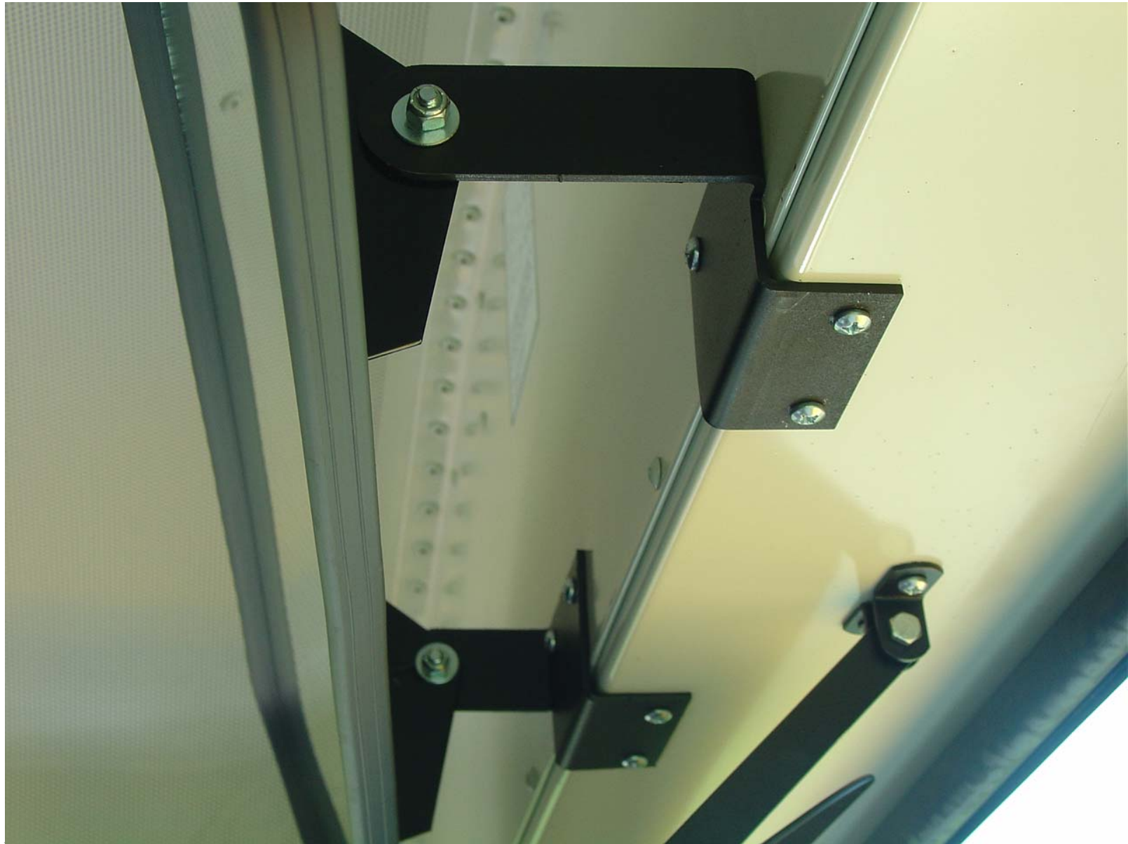
Photo 6 -Inside Rearview Mirror and Mounting
