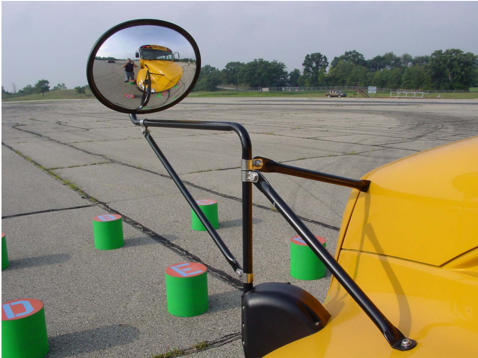
Photo 7 -Left Front Cross View Mirror and Mounting
