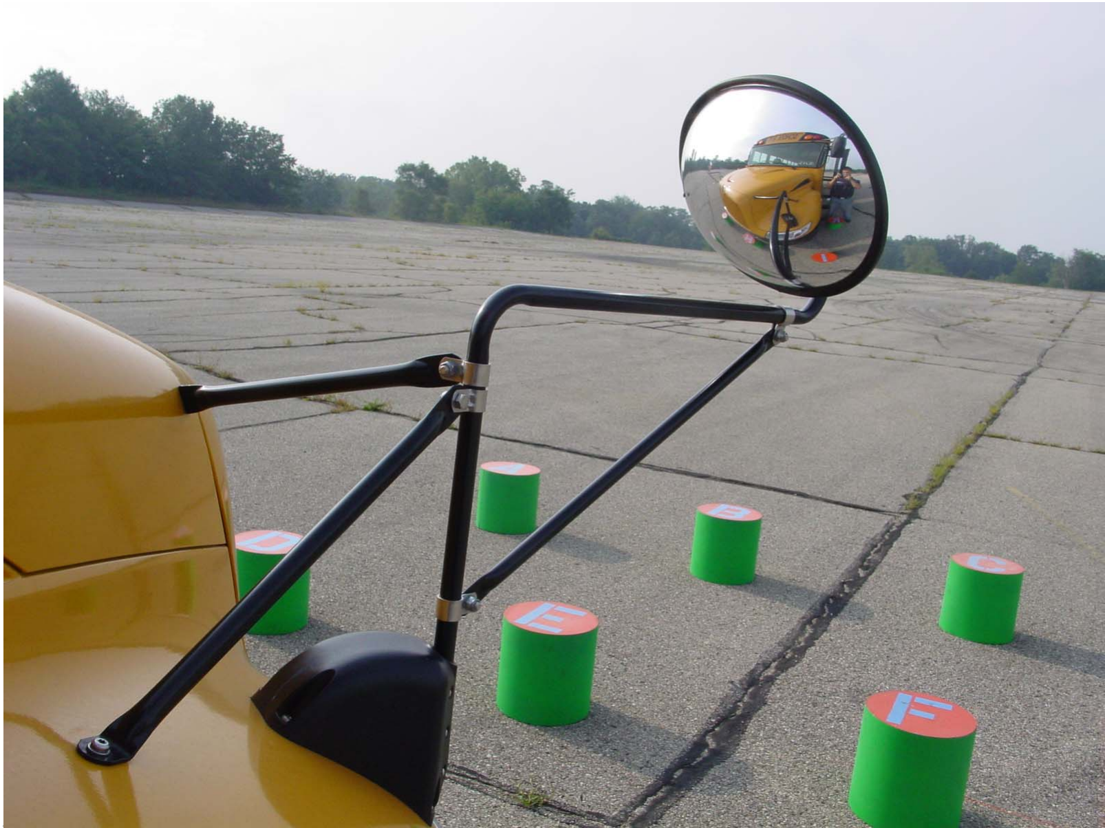
Photo 4 -Right Front Cross View Mirror and Mounting
