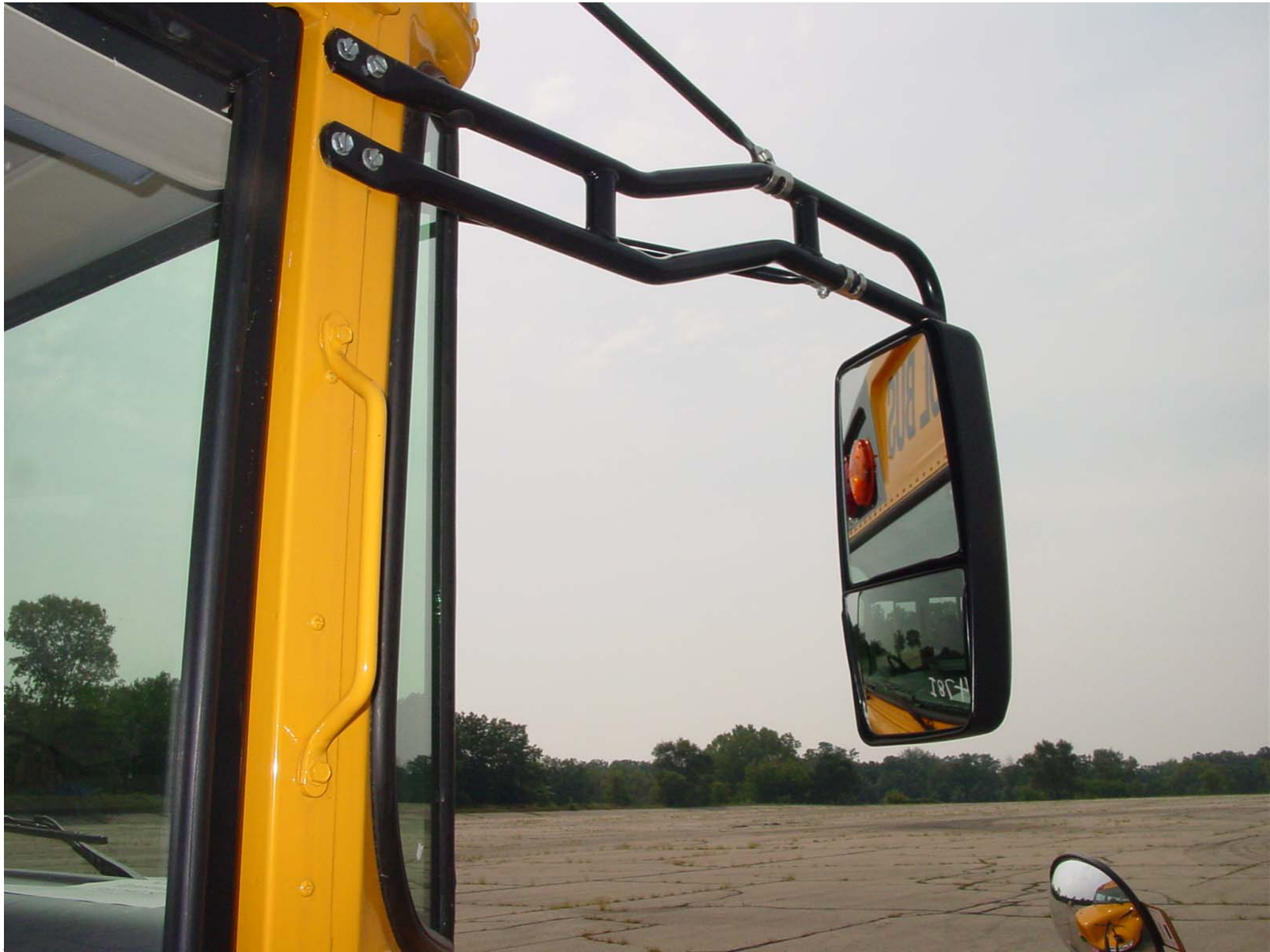
Photo 5 -Passenger Side Rearview Mirror and Mounting
