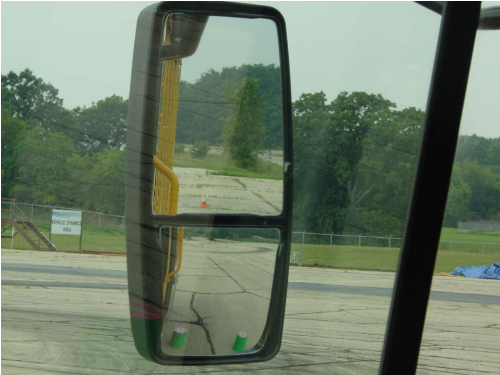
Photo 12 -Mirror #4 and #6 System A Field of View
