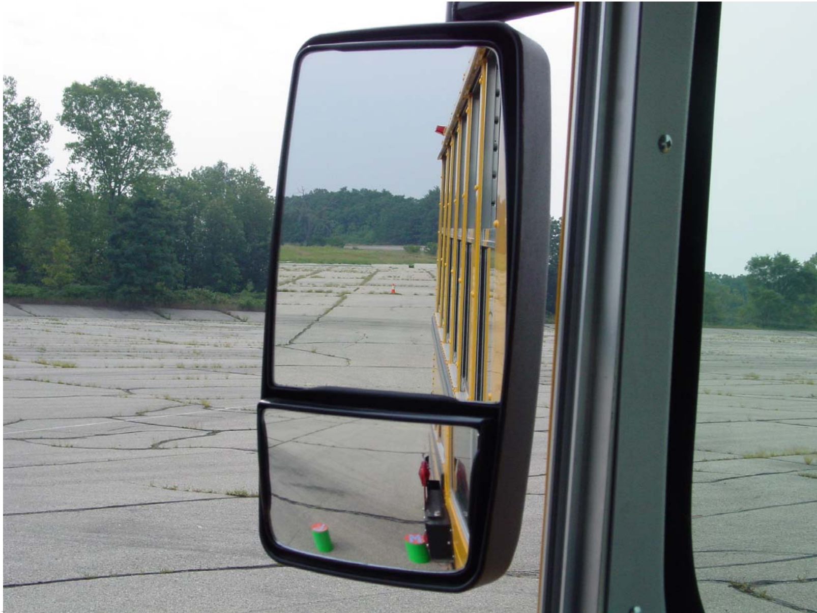
Photo 13 -Mirror #3 and #5 System A Field of View
