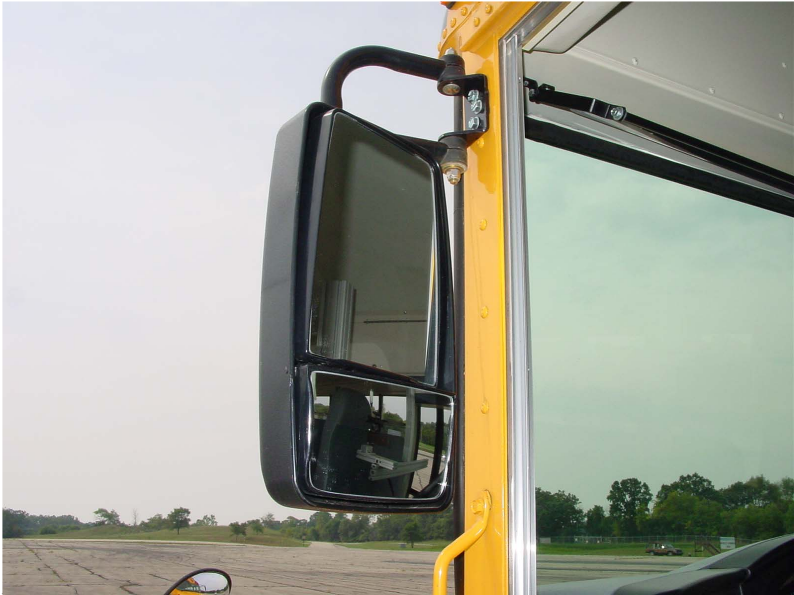
Photo 8 -Driver Side Rearview Mirror and Mounting
