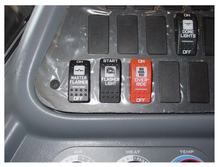
Photo 5 - Close Up View of the Switches That Allow Extension of the Stop Signal Arm(s)
