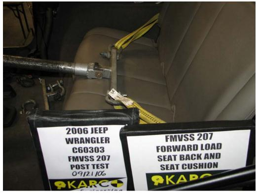
FIGURE 28. Forward Load on Seat Back, P4, Post-Test (Incorrect Sign)
