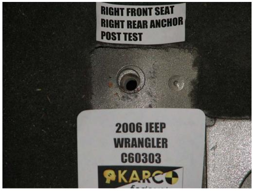
FIGURE 88. Floor Pan Anchor, P2, Post-Test
