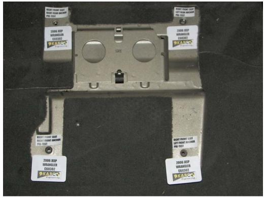
FIGURE 71. Floor Pan Anchors, P2 Overall, Pre-Test
