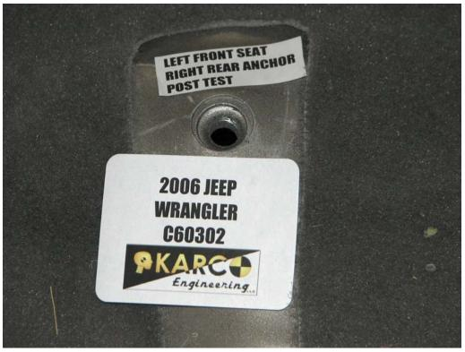
FIGURE 60. Floor Pan Anchor, P1, Post-Test
