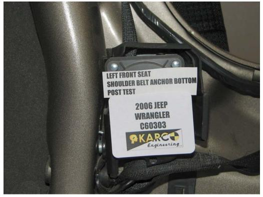
FIGURE 66. Shoulder Belt Anchor, P1, Post-Test
