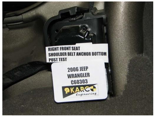
FIGURE 94. Shoulder Belt Anchor, P2, Post-Test
