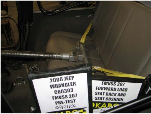
FIGURE 27. Forward Load on Seat Back, P4, Pre-Test (Incorrect Sign)
