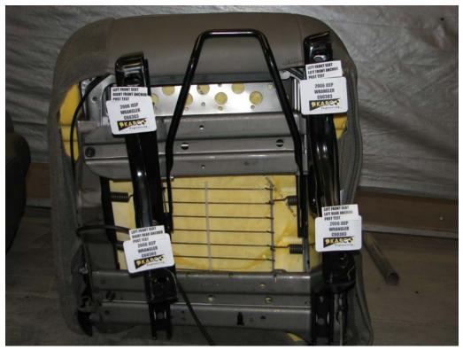
FIGURE 46. Seat Anchors, P1 Overall, Post-Test
