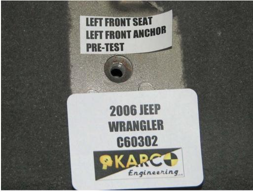
FIGURE 47. Floor Pan Anchor, P1, Pre-Test
