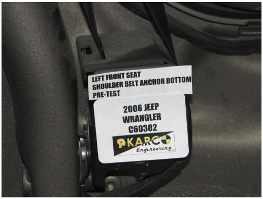
FIGURE 65. Shoulder Belt Anchor, P1, Pre-Test
