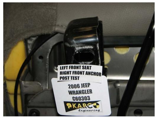
FIGURE 54. Seat Anchor, P1, Post-Test
