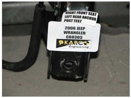
FIGURE 86. Seat Anchor, P2, Post-Test
