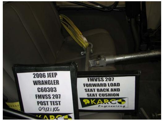
FIGURE 30. Forward Load on Seat Back, P3, Post-Test (Incorrect Sign)
