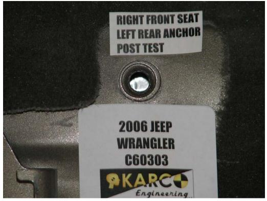
FIGURE 84. Floor Pan Anchor, P2, Post-Test
