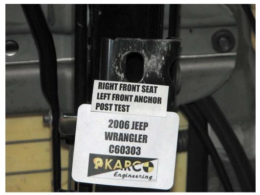
FIGURE 78. Seat Anchor, P2, Post-Test
