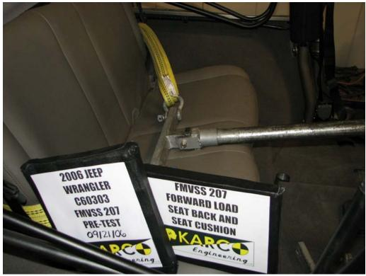
FIGURE 29. Forward Load on Seat Back, P3, Pre-Test (Incorrect Sign)
