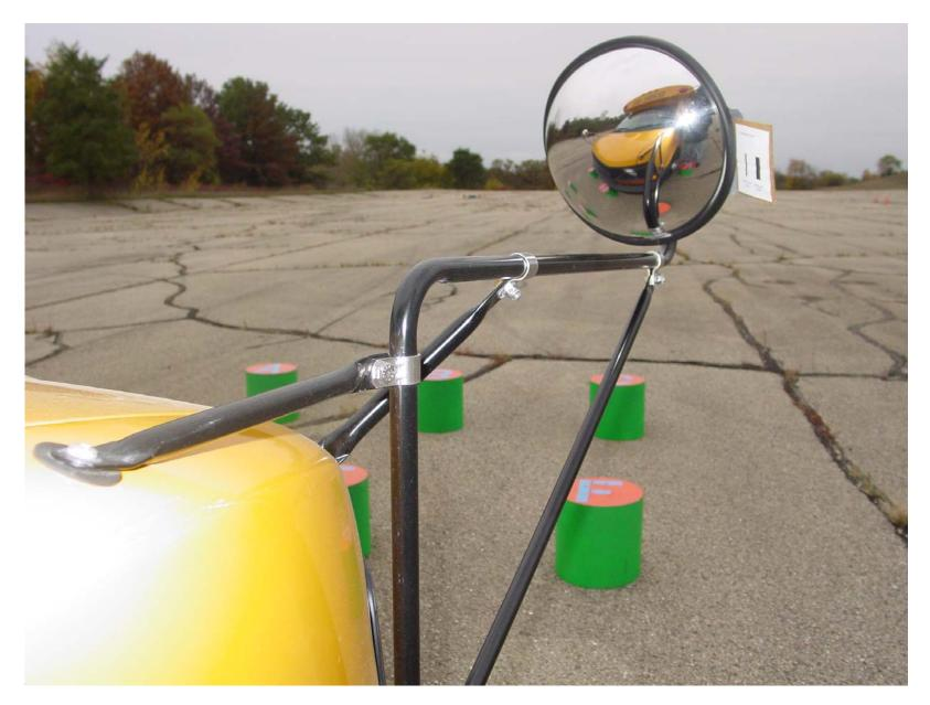
Test Vehicle:2006 Mid Bus Guide DWProcedure:FMVSS 111
