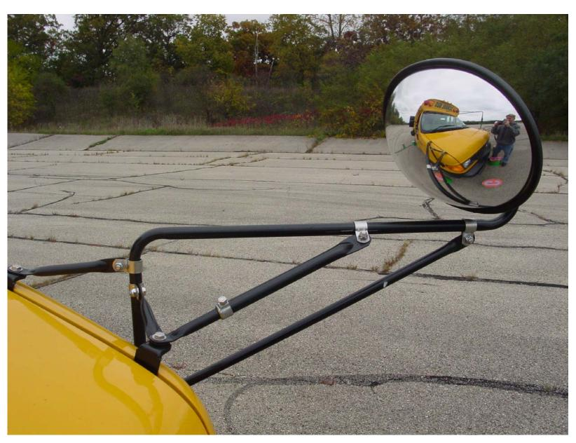
Photo 9 -Left Front Cross View Mirror and Mounting
