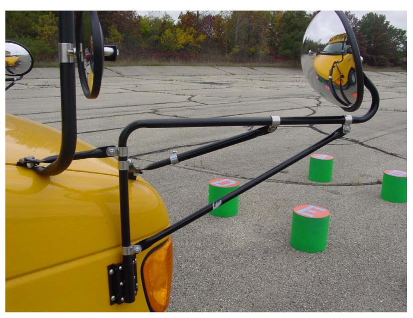
Photo 6 -Right Front Cross View Mirror and Mounting
