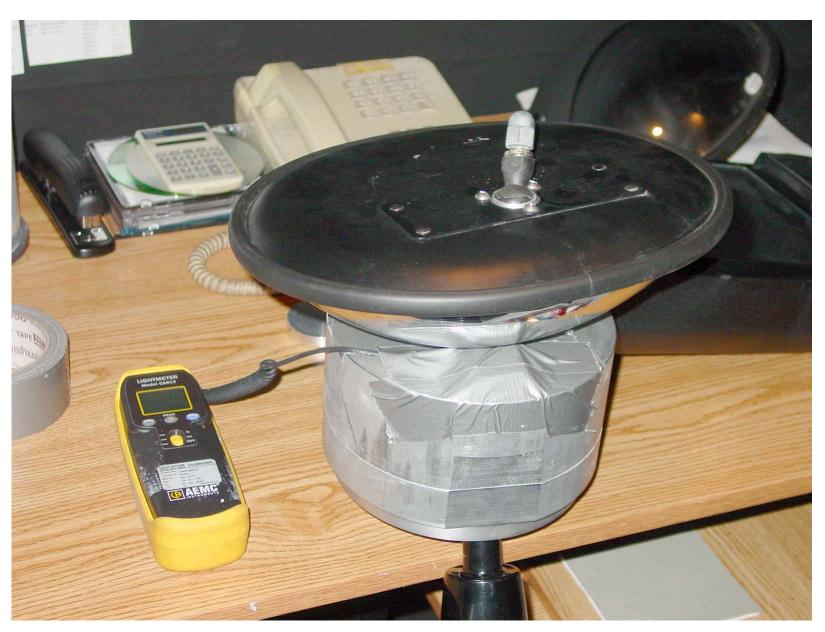
Photo 22 -Reflectance Test Set-up
