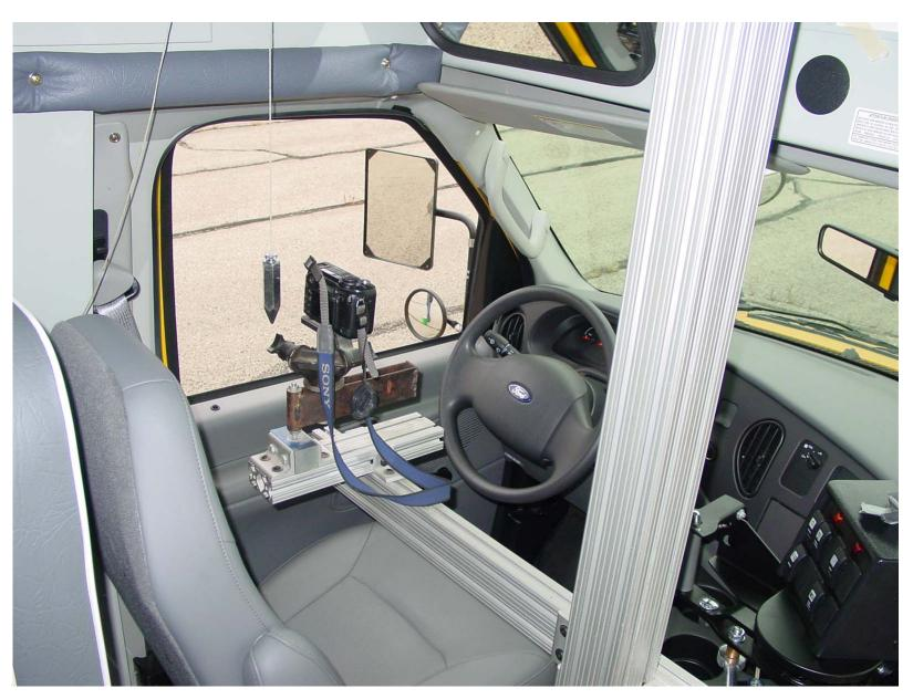
Photo 11 -Field of View Instrument Setup
