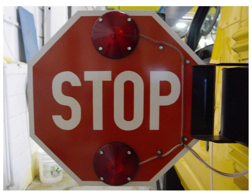
Photo 6- Back Close Up View of Stop Signal Arm
