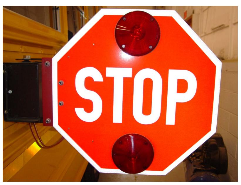
Photo 5- Front Close Up View of Stop Signal Arm
