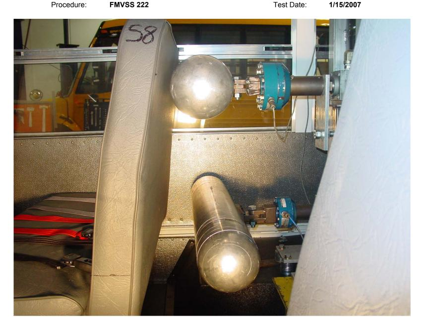
Pre-Test of Seat Back S8 Force Deflection Forward Test
