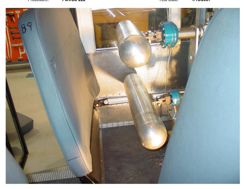
Post-Test of Barrier B9 Force Deflection Forward Test
