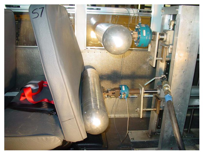
Post-Test of Seat Back S7 Force Deflection Forward Test
