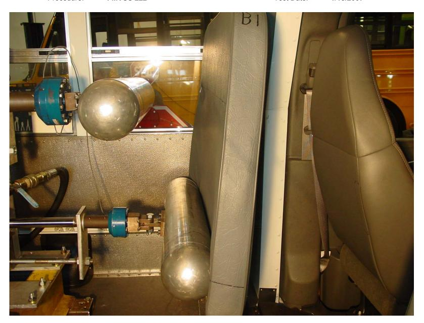
Post-Test of Barrier B1 Force Deflection Forward Test View 2
