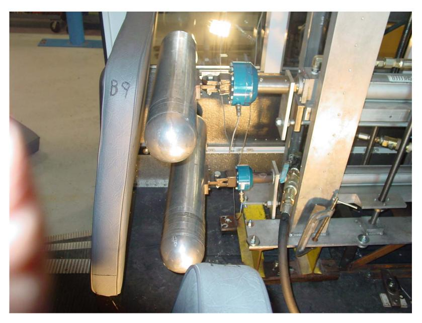
Pre-Test of Barrier B9 Force Deflection Forward Test
