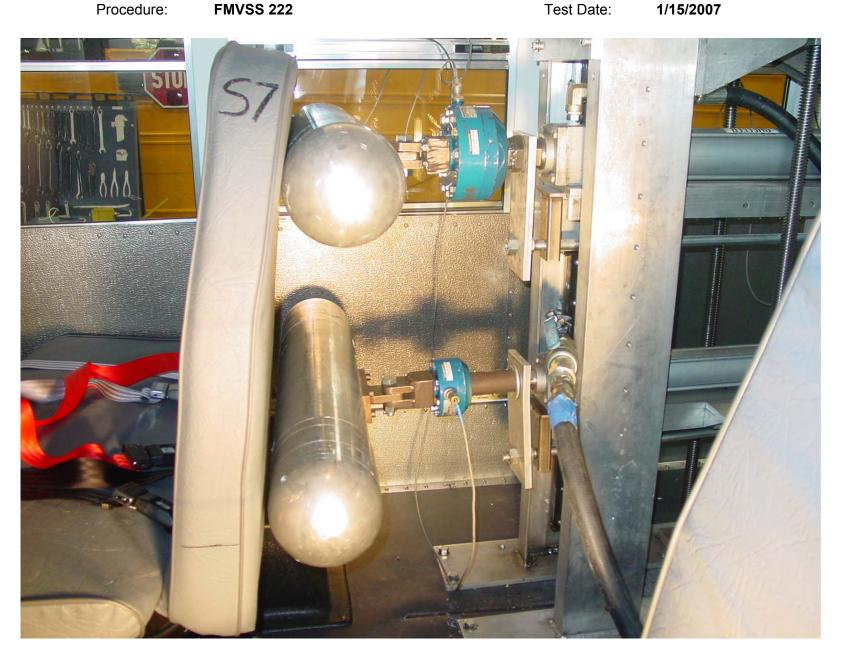
Pre-Test of Seat Back S7 Force Deflection Forward Test
