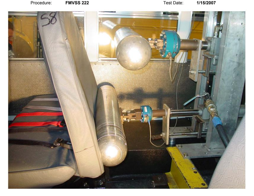
Post-Test of Seat Back S8 Force Deflection Forward Test
