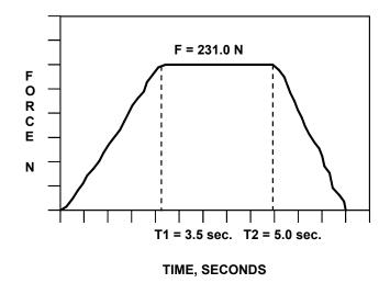
F must be 5 x Cushion Weight; t1 and t2 must be according to the following expressions: T1=>1 sec., <5 sec., t2=t1+5 sec., +0 sec. and -0.10 sec.
