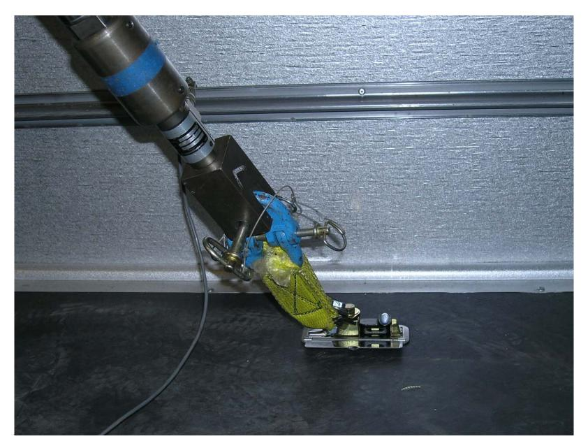
Post-Test of Wheelchair Anchorage W8.5 Left Front Type A Load Test
