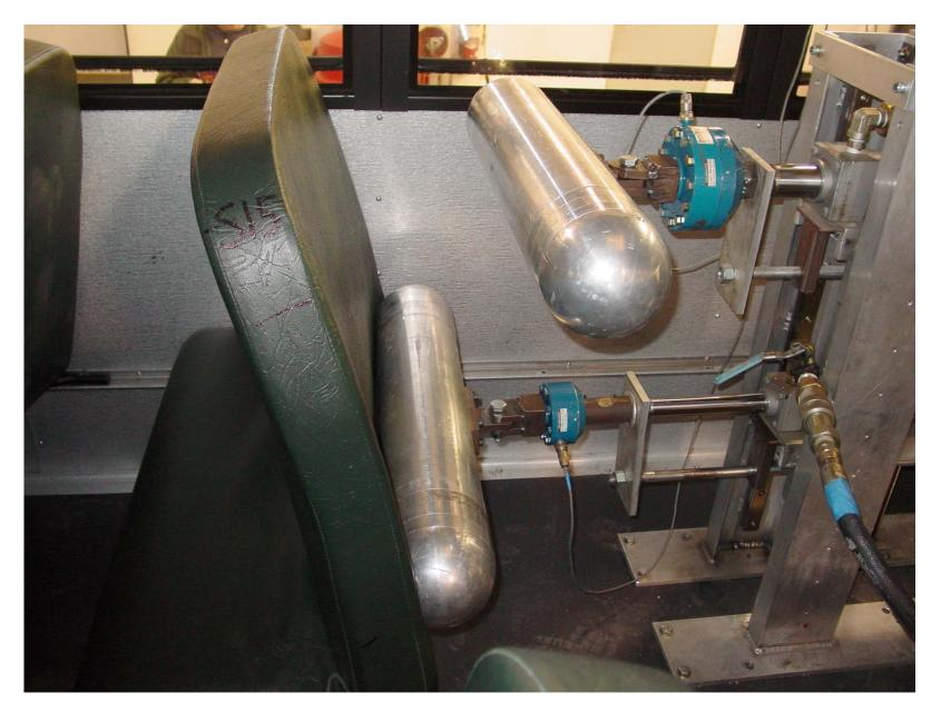
Post-Test of Seat Back S15 Force Deflection Forward Test
