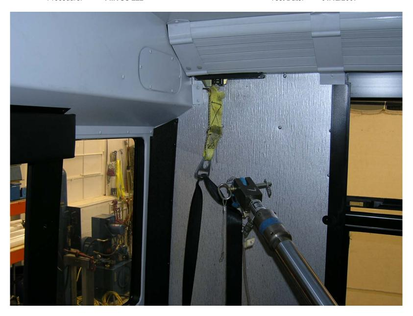
Post-Test of Wheelchair Anchorage W8.5 Upper Torso Type D Load Test
