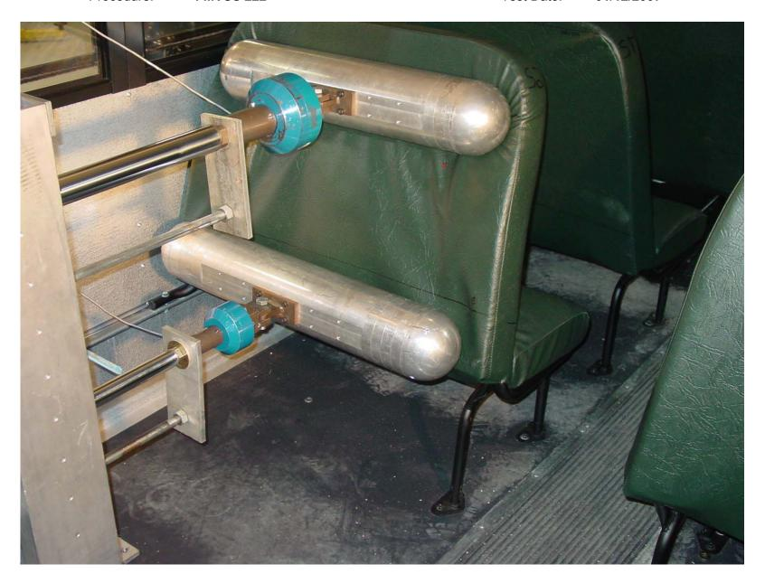
Test (In Progress) of Seat Back S2 Force Deflection Forward Test
