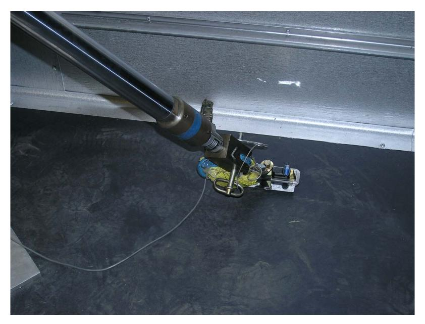
Pre-Test of Wheelchair Anchorage W8.5 Left Front Type A Load Test
