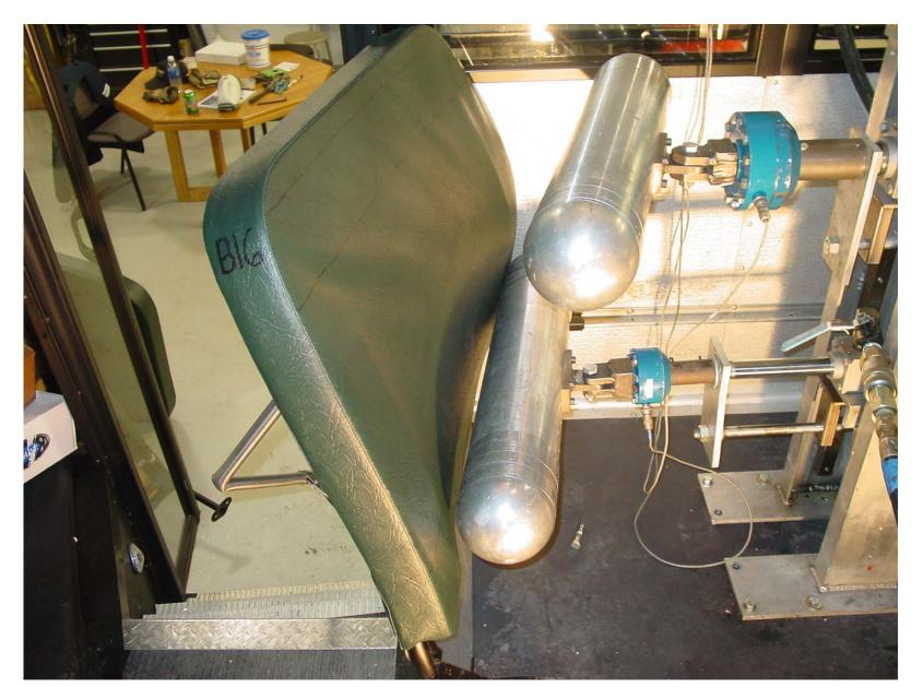
Post-Test of Barrier B16 Force Deflection Forward Test
