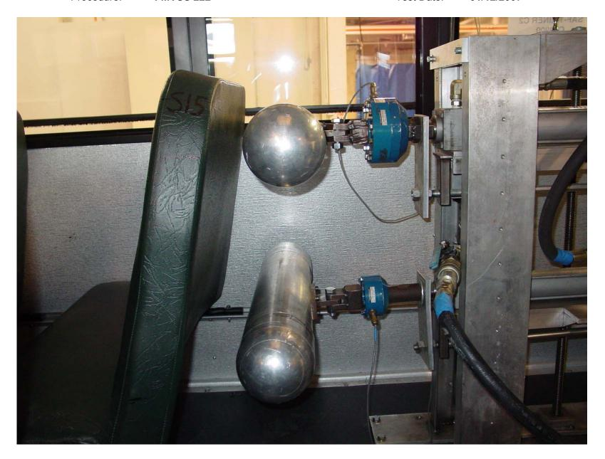
Pre-Test of Seat Back S15 Force Deflection Forward Test
