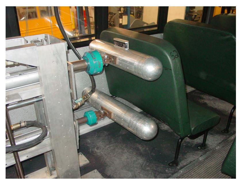
Pre-Test of Seat Back S2 Force Deflection Forward Test
