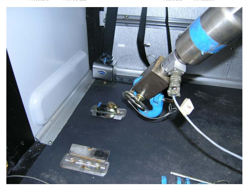
Pre-Test of Wheelchair Anchorage W8.5 Left Rear Type C Load Test
