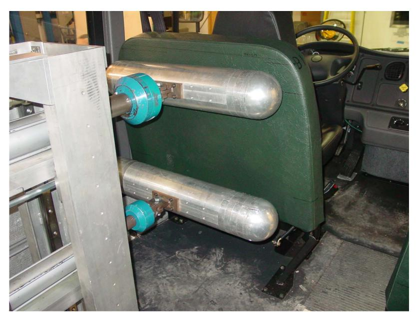
Pre-Test of Barrier B1 Force Deflection Forward Test
