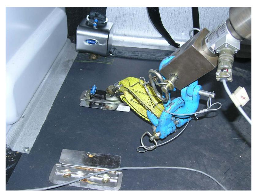
Post-Test of Wheelchair Anchorage W8.5 Left Rear Type C Load Test
