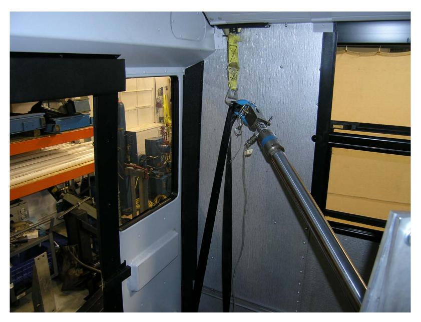
Pre-Test of Wheelchair Anchorage W8.5 Upper Torso Type D Load Test
