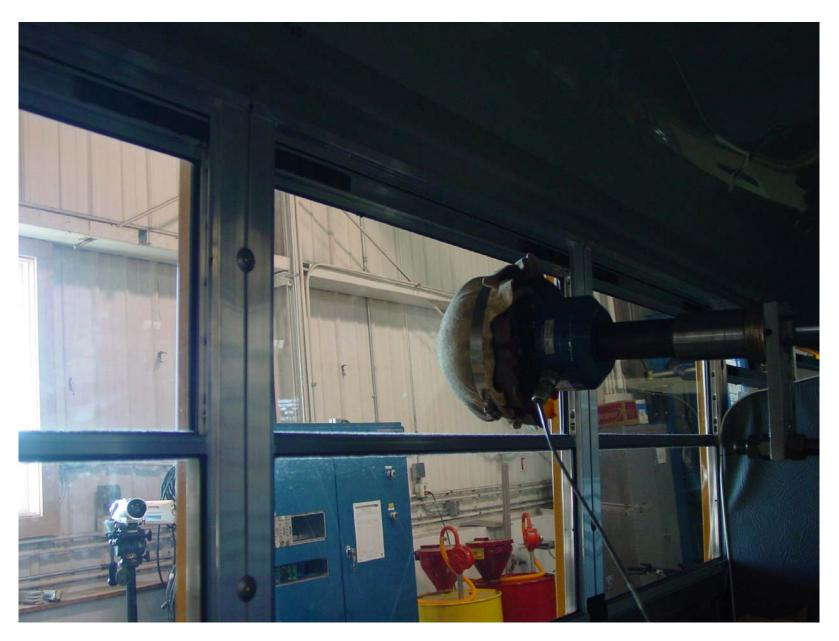
Retention Test of Left Side Window (Post-Test)
