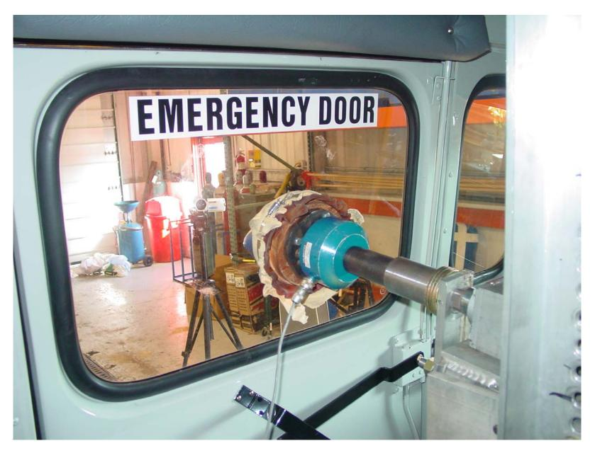
Retention Test of Rear Door Window (Post-Test)
