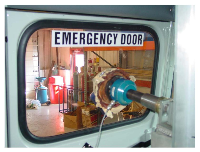
Retention Test of Rear Door Window (Pre-Test)
