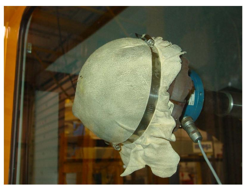
Retention Test of Rear Door Window (Pre-Test)
