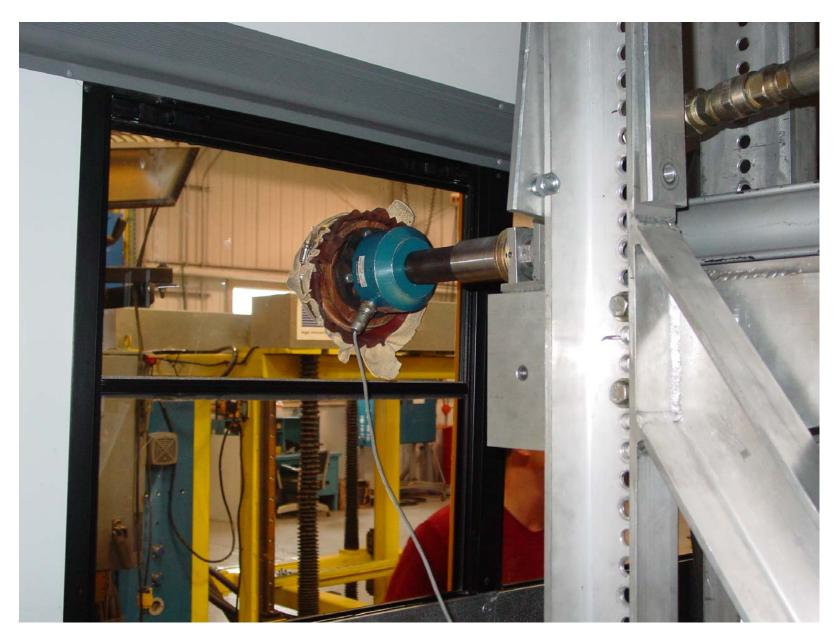
Retention Test of Left Side Window (Pre-Test)
