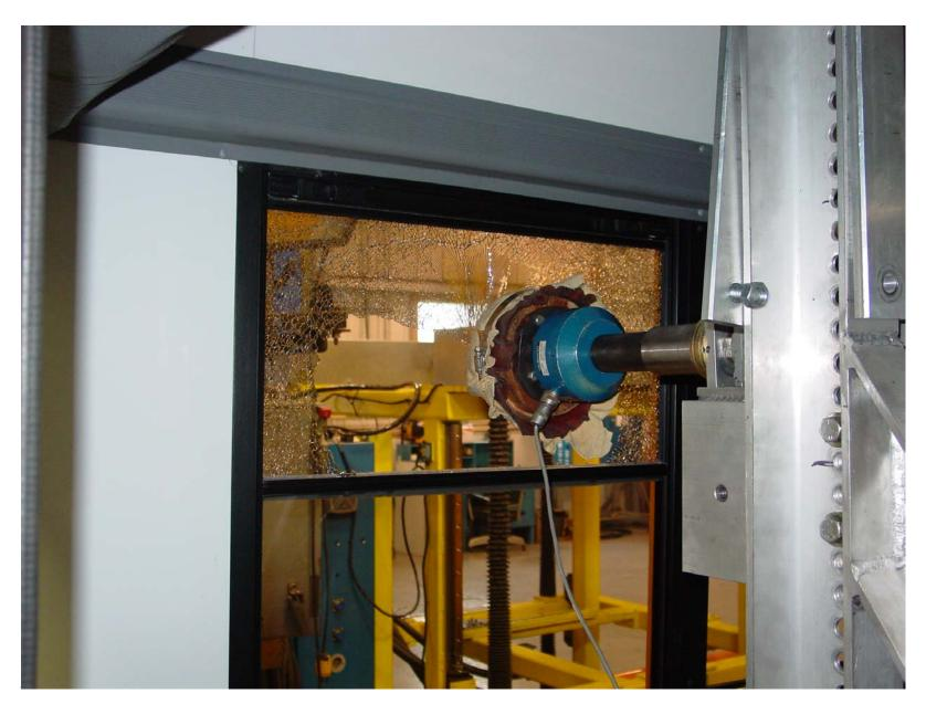
Retention Test of Left Side Window (Post-Test)
