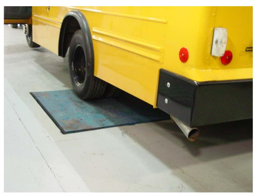
Vehicle on Scales Doing Measurement of Rear Axle Loads
