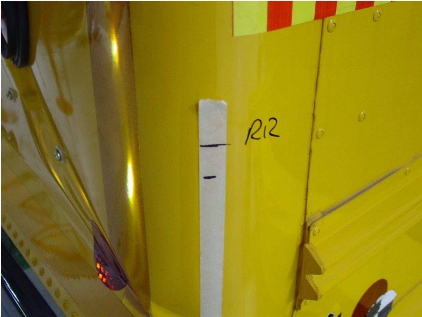
Back-up Roof Deflection Measuring Device at RR Corner of Bus at Full Load
