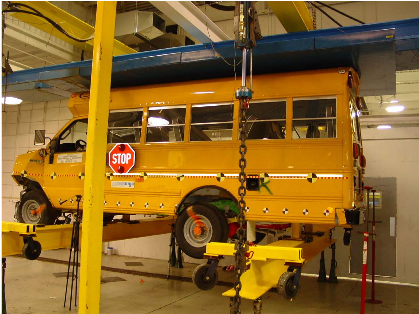
Loading Device Placed Against Bus Roof At Start of Test
