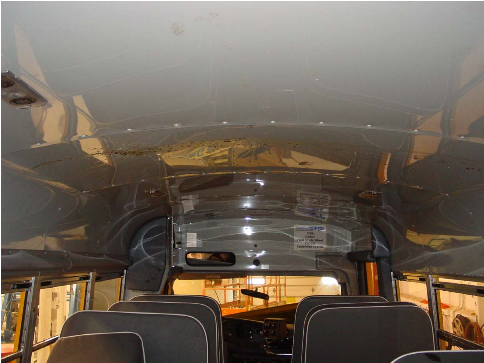
Roof, Before Application of Loading Device, Viewed From Bus Interior
