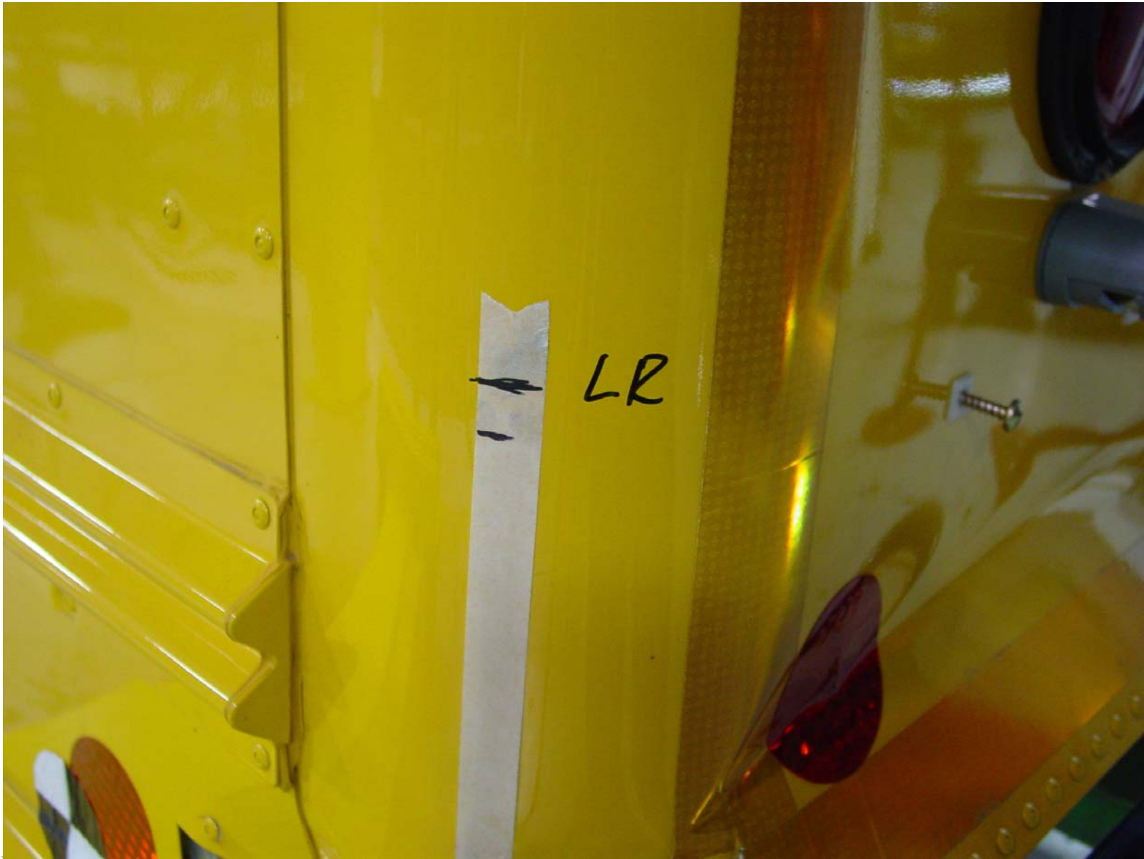
Back-up Roof Deflection Measuring Device at LR Corner of Bus at Full Load
