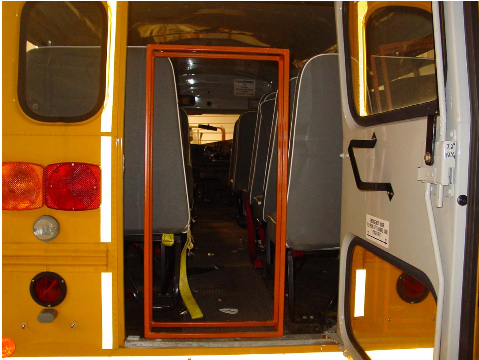
Exit Opened After Roof Loading is Attained with Parallelepiped in Place
