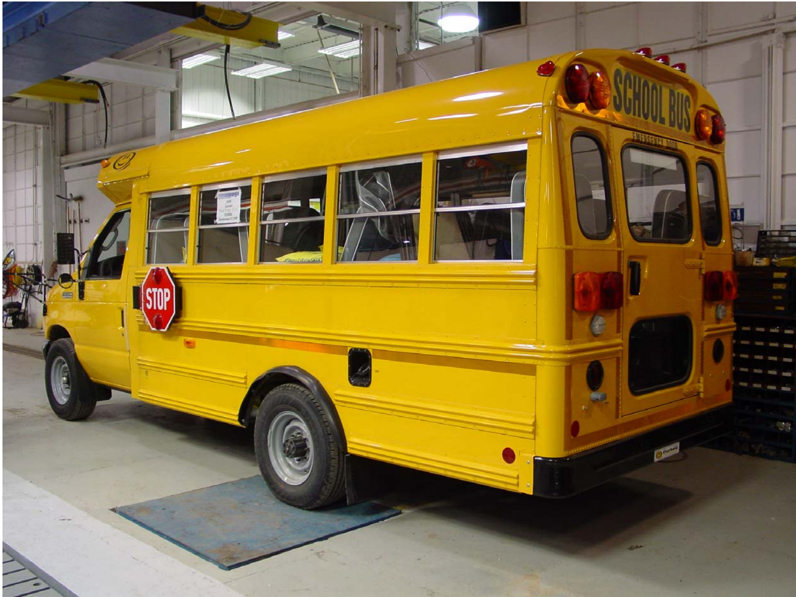
School Bus Rear Axle Being Weighed (as received by MGA)
