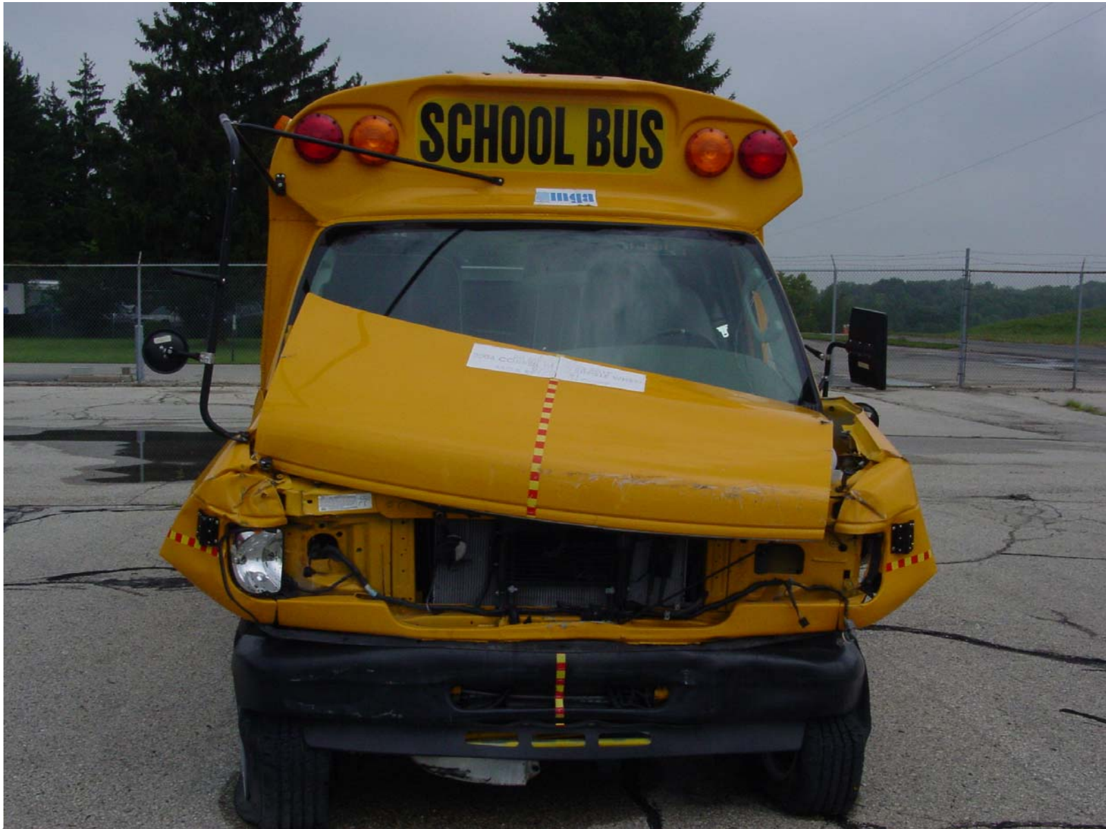
Frontal View of School Bus After Testing (front structure damage from FMVSS 301)
