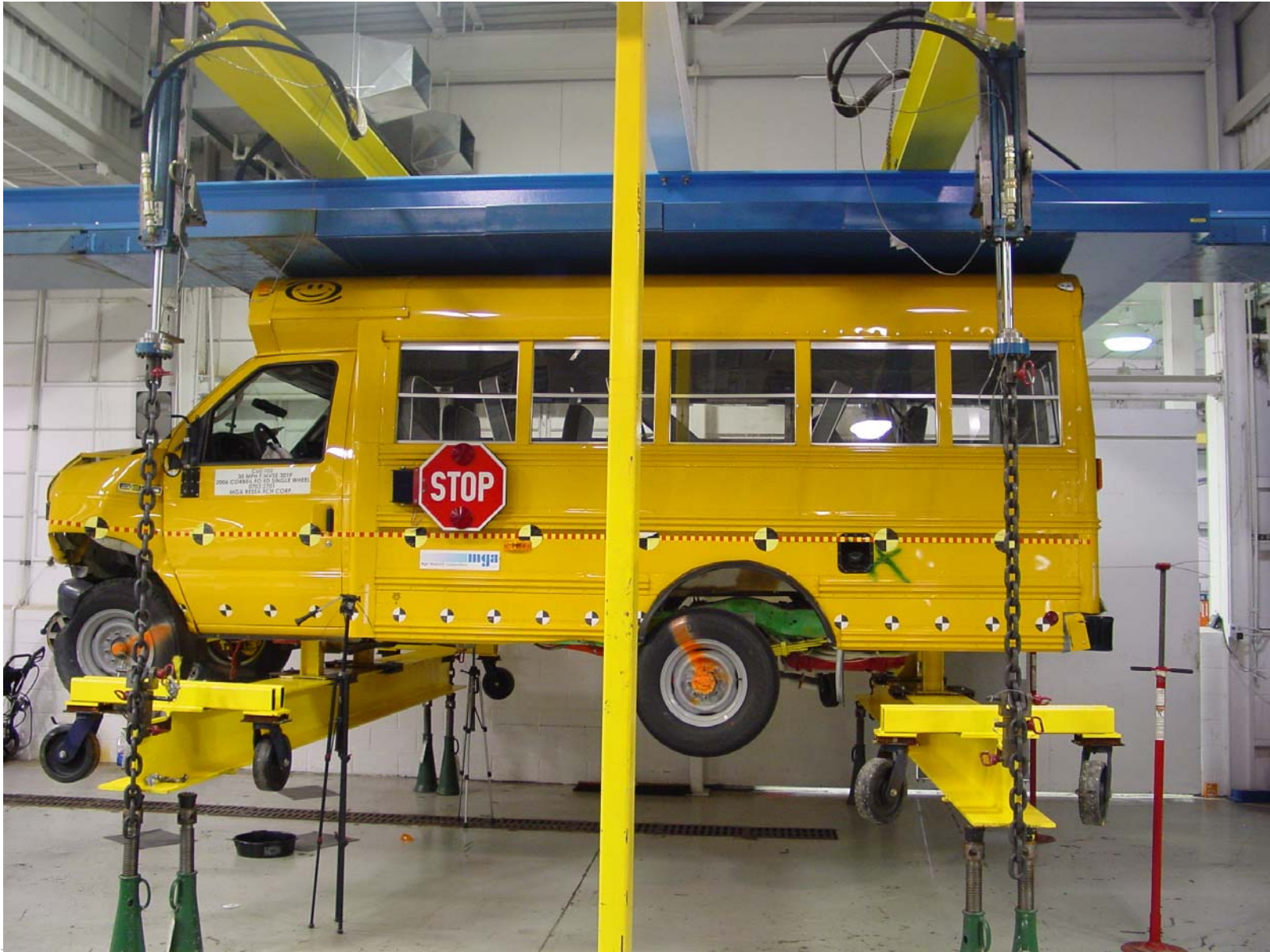
Loading Device Placed Against Bus Roof at Maximum Load
