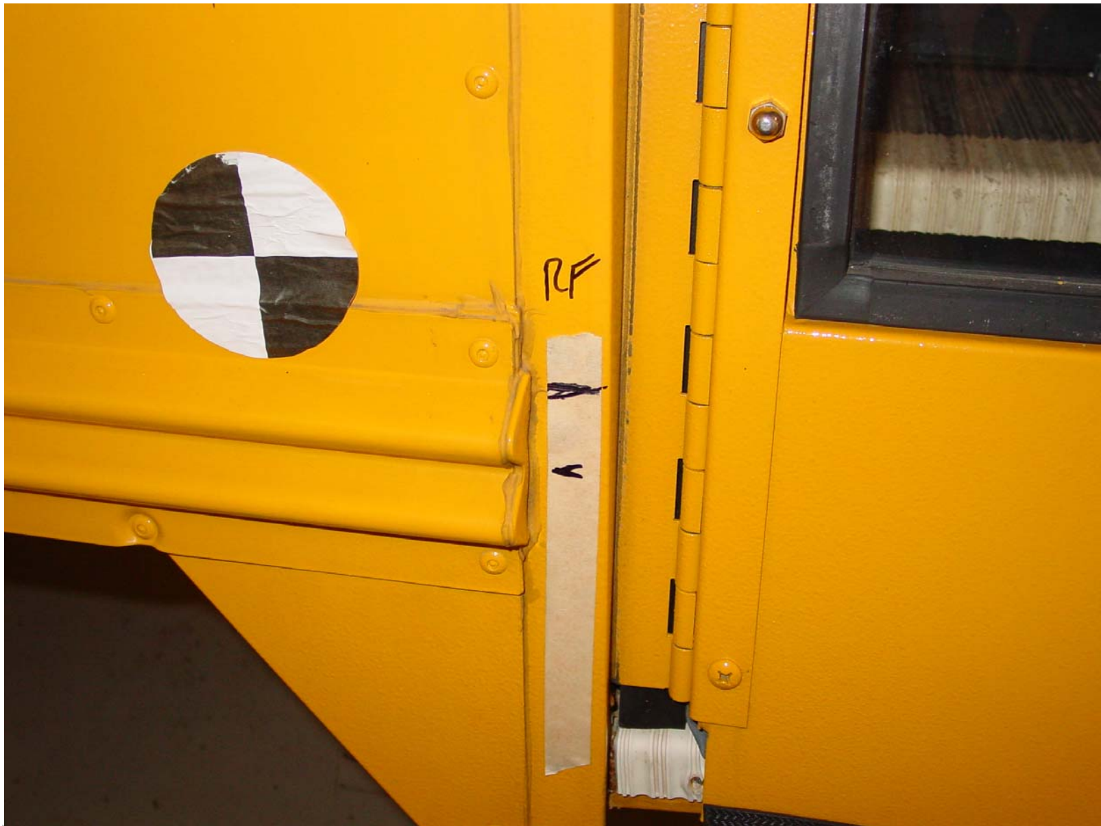
Back-up Roof Deflection Measuring Device at RF Corner of Bus at Full Load
