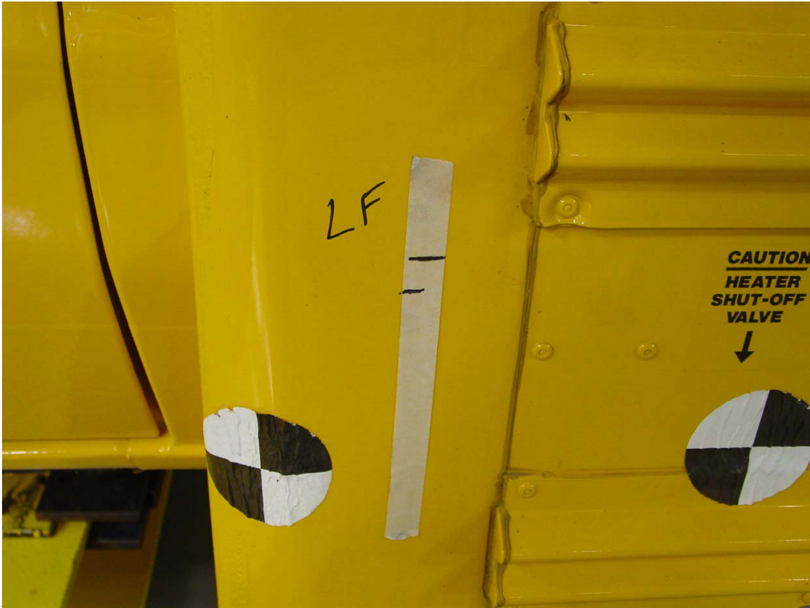
Back-up Roof Deflection Measuring Device at LF Corner of Bus at Full Load
