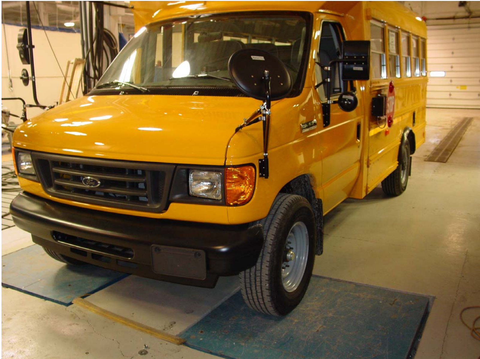
School Bus Front Axle Being Weighed (as received by MGA)
