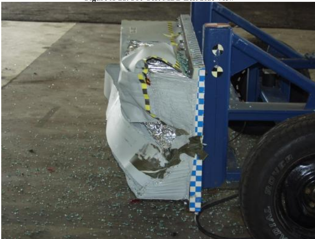
Figure A-22: Post-Test MDB Left Side View
