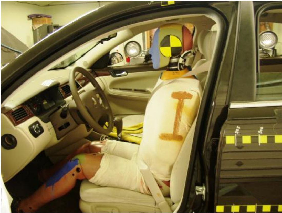
Figure A-29: Pre-Test Impact Side View of SID HIII with Door Open
