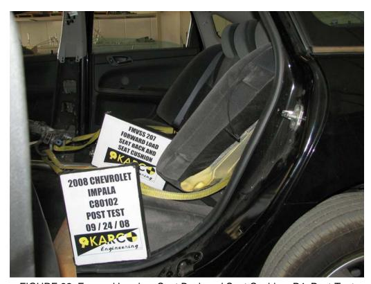
FIGURE 32. Forward Load on Seat Back and Seat Cushion, P4, Post-Test
