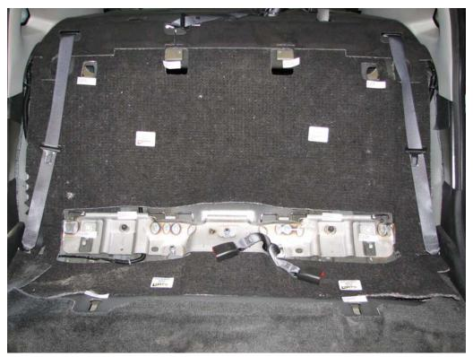
FIGURE 95. Floor Pan Anchors, P3 & P4 Overall, Pre-Test
