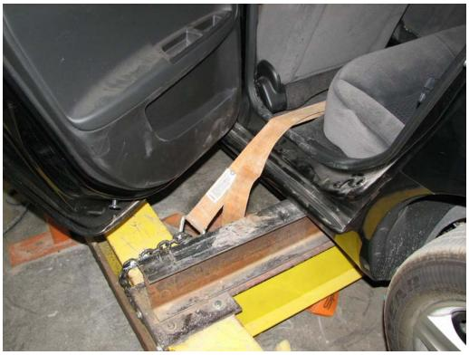
FIGURE 10. Vehicle Mounted in Test Fixture
