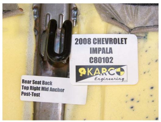
FIGURE 110. Seat Back Anchor, P3, Post-Test
