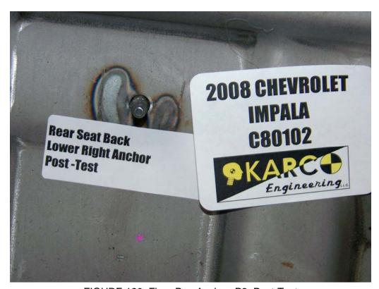
FIGURE 120. Floor Pan Anchor, P3, Post-Test
