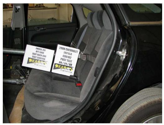
FIGURE 36. Aft Load on Seat Back and Seat Cushion, P4, Post-Test
