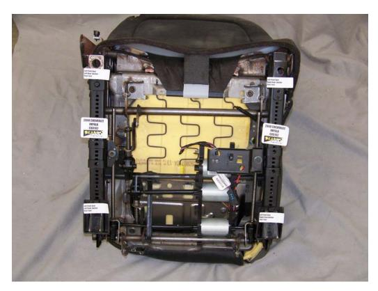
FIGURE 42. Seat Anchors, P1 Overall, Post-Test
