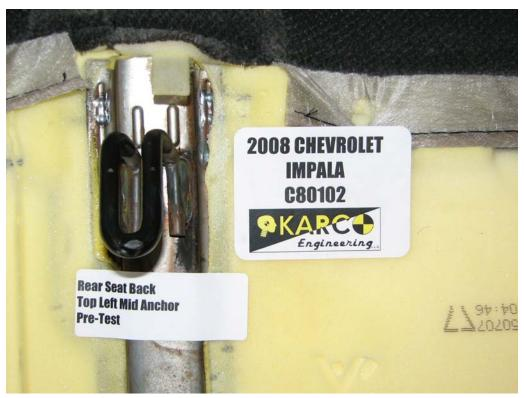
FIGURE 105. Seat Back Anchor, P4, Pre-Test
