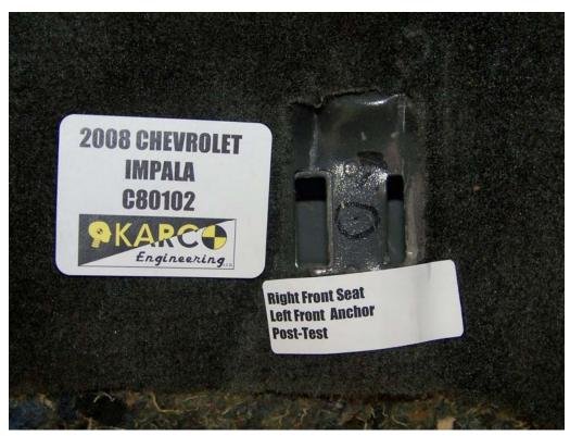
FIGURE 72. Floor Pan Anchor, P2, Post-Test
