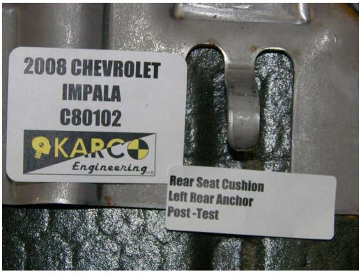
FIGURE 134. Floor Pan Anchor, P4, Post-Test
