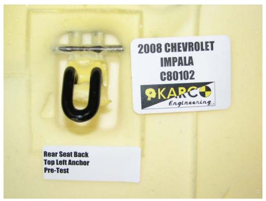
FIGURE 101. Seat Back Anchor, P4, Pre-Test
