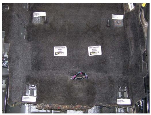
FIGURE 40. Floor Pan Anchors, P1 Overall, Post-Test
