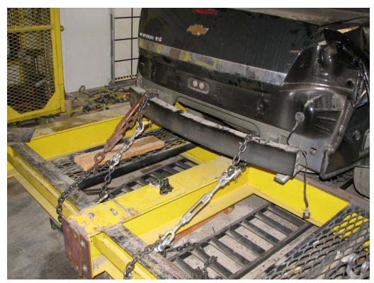
FIGURE 9. Vehicle Mounted in Test Fixture
