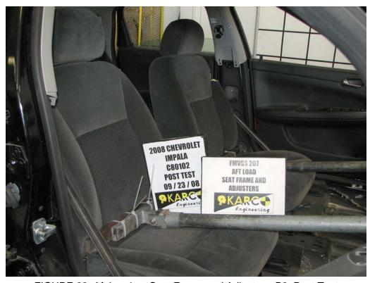
FIGURE 22. Aft Load on Seat Frame and Adjusters, P2, Post-Test
