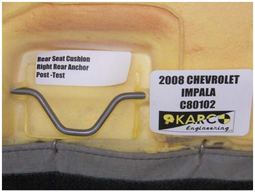
FIGURE 140. Seat Cushion Anchor, P3, Post-Test
