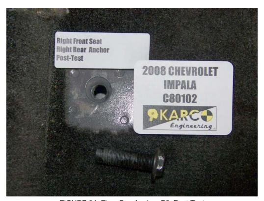
FIGURE 84. Floor Pan Anchor, P2, Post-Test
