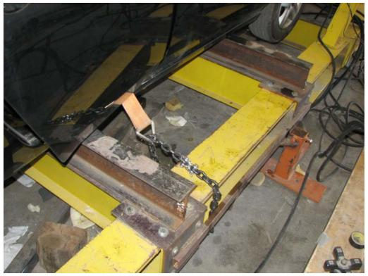
FIGURE 8. Vehicle Mounted in Test Fixture
