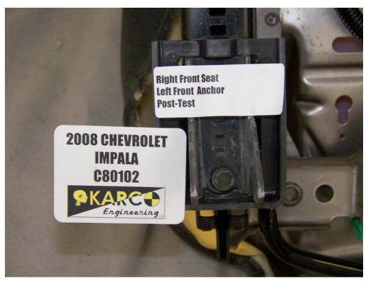
FIGURE 74. Seat Anchor, P2, Post-Test
