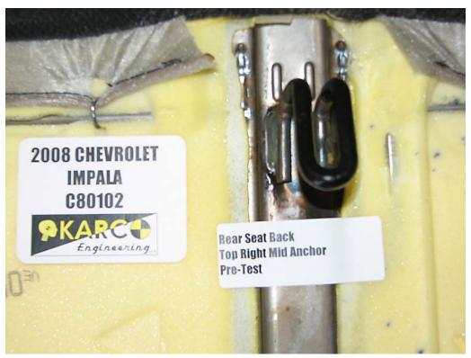
FIGURE 109. Seat Back Anchor, P3, Pre-Test
