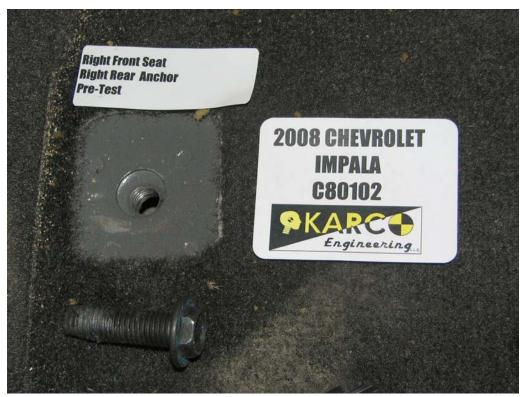
FIGURE 83. Floor Pan Anchor, P2, Pre-Test
