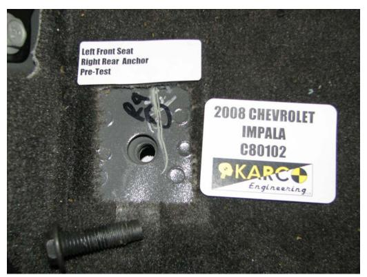
FIGURE 55. Floor Pan Anchor, P1, Pre-Test
