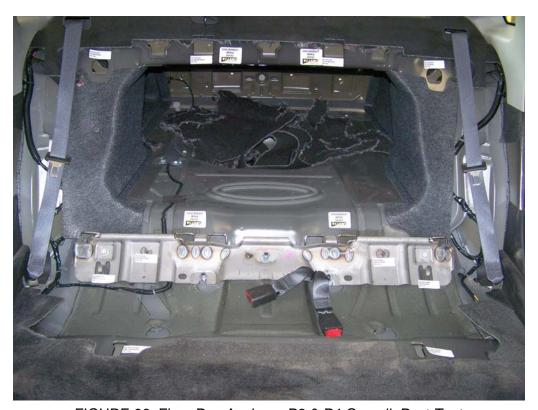
FIGURE 96. Floor Pan Anchors, P3 & P4 Overall, Post-Test
