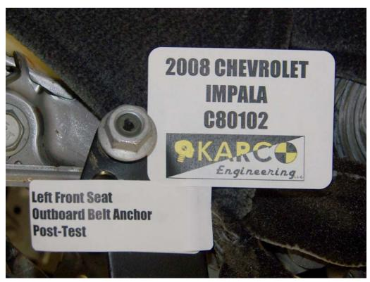
FIGURE 64. Belt Anchor, P1, Post-Test
