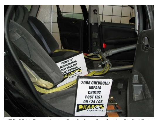
FIGURE 34. Forward Load on Seat Back and Seat Cushion, P3, Post-Test
