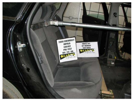
FIGURE 29. Aft Moment on Seat Back, P3, Pre-Test
