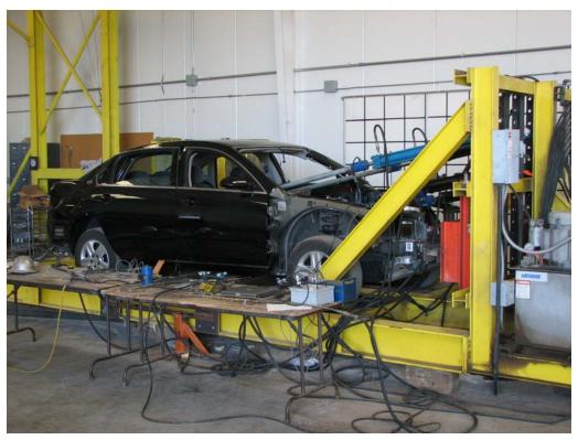
FIGURE 7. Vehicle Mounted in Test Fixture
