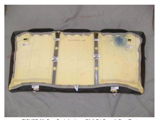
FIGURE 98. Seat Back Anchors, P3 & P4 Overall, Post-Test
