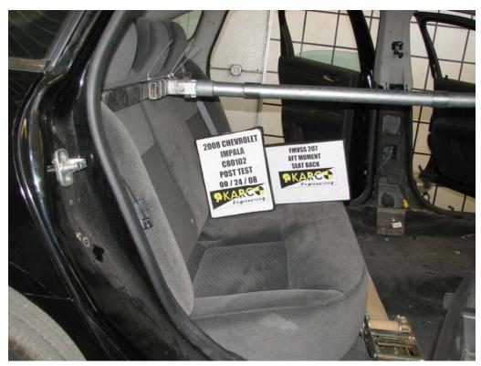
FIGURE 30. Aft Moment on Seat Back, P3, Post-Test
