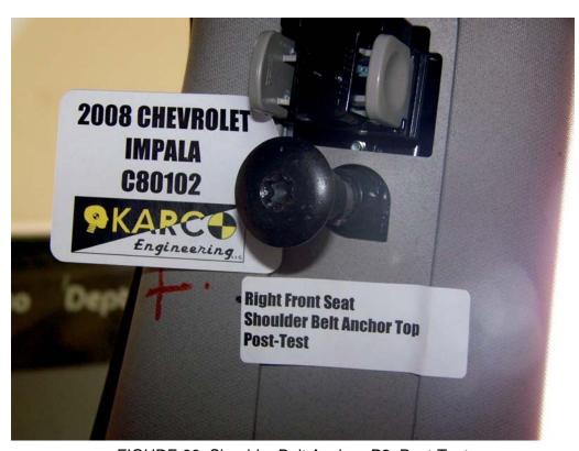
FIGURE 88. Shoulder Belt Anchor, P2, Post-Test
