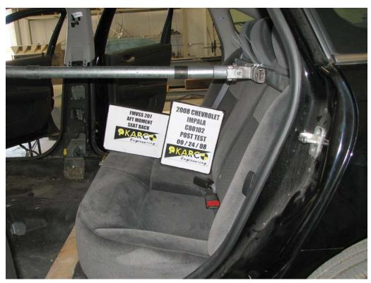
FIGURE 28. Aft Moment on Seat Back, P4, Post-Test
