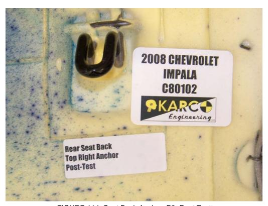
FIGURE 114. Seat Back Anchor, P3, Post-Test
