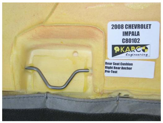
FIGURE 139. Seat Cushion Anchor, P3, Pre-Test
