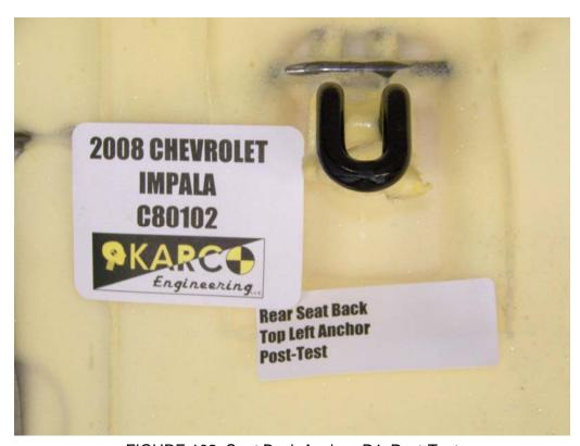
FIGURE 102. Seat Back Anchor, P4, Post-Test
