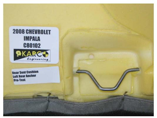
FIGURE 135. Seat Cushion Anchor, P4, Pre-Test
