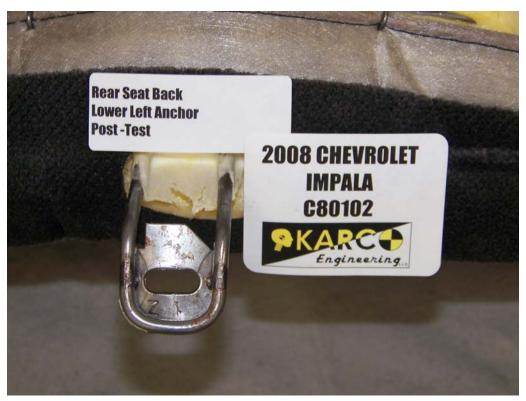
FIGURE 118. Seat Back Anchor, P4, Post-Test
