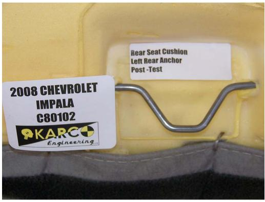
FIGURE 136. Seat Cushion Anchor, P4, Post-Test
