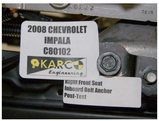
FIGURE 94. Belt Anchor, P2, Post-Test
