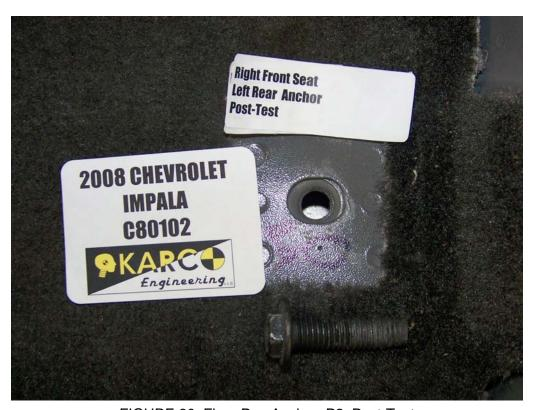
FIGURE 80. Floor Pan Anchor, P2, Post-Test
