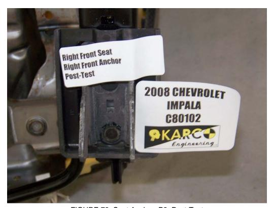
FIGURE 78. Seat Anchor, P2, Post-Test
