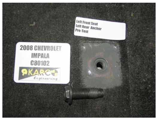
FIGURE 51. Floor Pan Anchor, P1, Pre-Test
