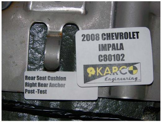
FIGURE 138. . Floor Pan Anchor, P3, Post-Test
