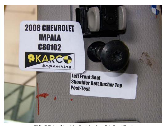
FIGURE 60. Shoulder Belt Anchor, P1, Post-Test
