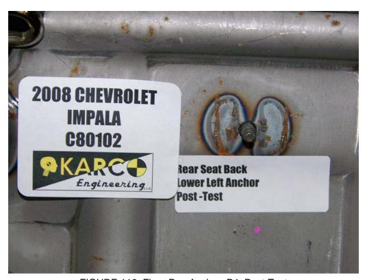
FIGURE 116. Floor Pan Anchor, P4, Post-Test
