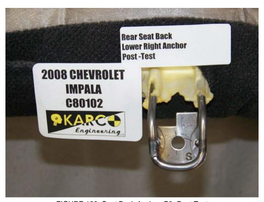
FIGURE 122. Seat Back Anchor, P3, Post-Test
