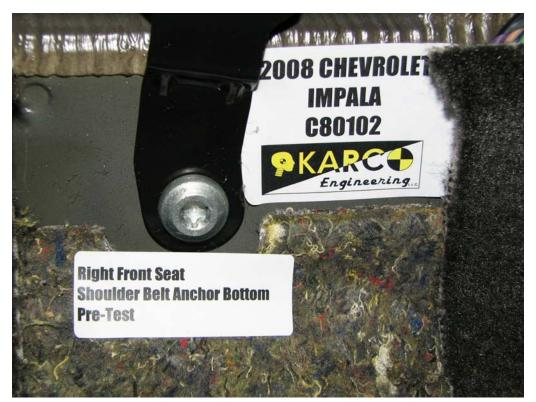
FIGURE 89. Shoulder Belt Anchor, P2, Pre-Test
