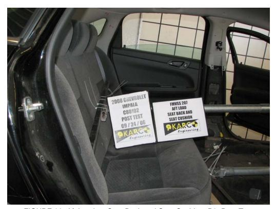
FIGURE 38. Aft Load on Seat Back and Seat Cushion, P3, Post-Test
