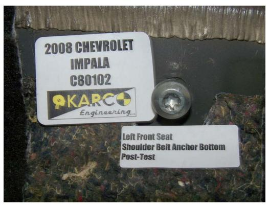
FIGURE 62. Shoulder Belt Anchor, P1, Post-Test
