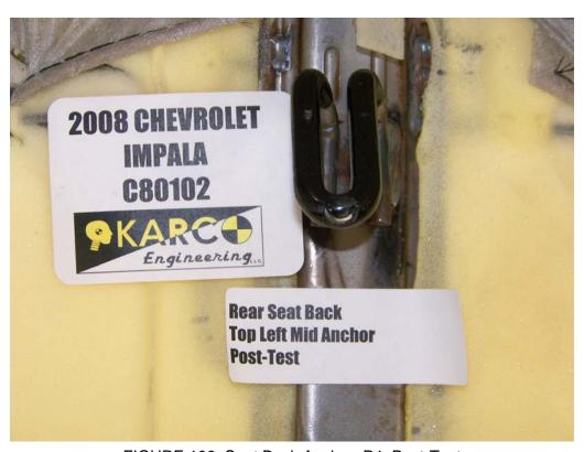
FIGURE 106. Seat Back Anchor, P4, Post-Test
