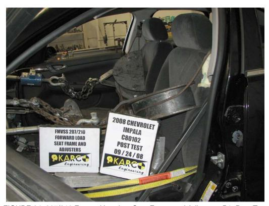
FIGURE 24. 207/210 Forward Load on Seat Frame and Adjusters, P1, Post-Test
