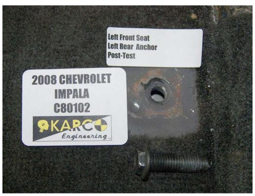
FIGURE 52. Floor Pan Anchor, P1, Post-Test
