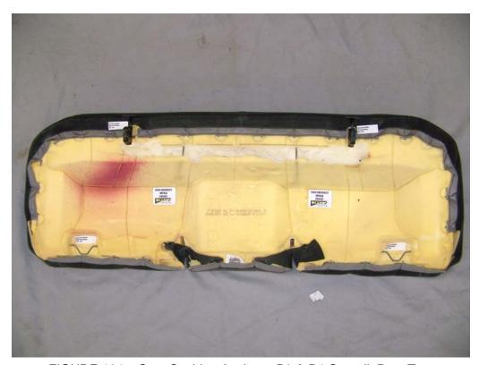
FIGURE 124. . Seat Cushion Anchors, P3 & P4 Overall, Post-Test
