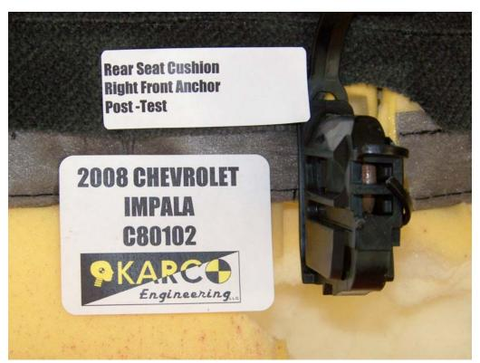
FIGURE 132. Seat Cushion Anchor, P3, Post-Test
