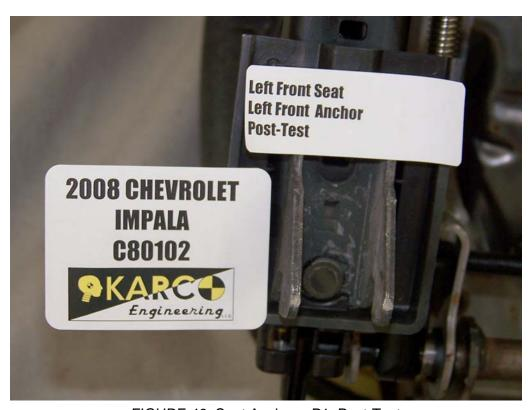
FIGURE 46. Seat Anchors, P1, Post-Test
