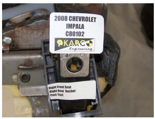
FIGURE 86. Seat Anchor, P2, Post-Test
