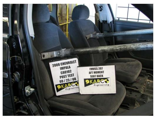
FIGURE 14. Aft Moment on Seat Back, P2, Post-Test
