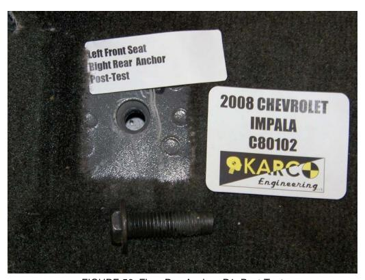
FIGURE 56. Floor Pan Anchor, P1, Post-Test
