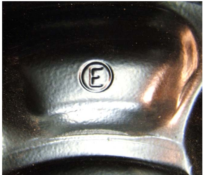
LEFT REAR RIM SHOWING LETTER DESIGNATION FOR SOURCE OF PUBLISHED DIMENSIONS, SIZE, DOT SYMBOL, MANUFACTURER'S SYMBOL, DATE OF MANUFACTURE, AND OTHER RIM MARKINGS
