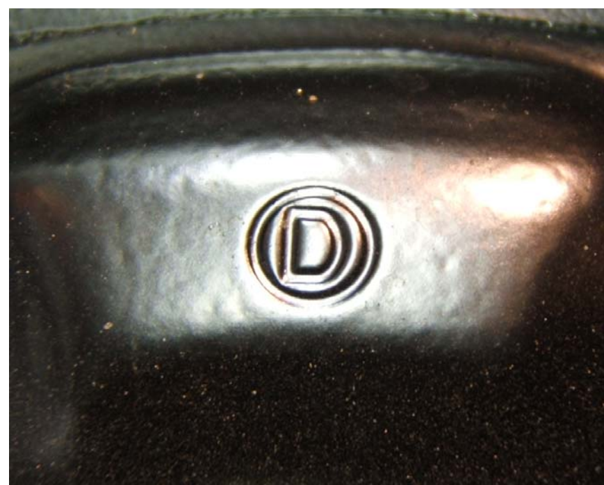
RIGHT FRONT RIM SHOWING LETTER DESIGNATION FOR SOURCE OF PUBLISHED DIMENSIONS, SIZE, DOT SYMBOL, MANUFACTURER'S SYMBOL, DATE OF MANUFACTURE, AND OTHER RIM MARKINGS
