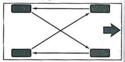
When rotating the vehicle's tires, always use the correct rotation pattern shown here.
