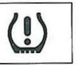
For vehicles with a tire pressure light, this light comes on briefly when the engine is started.
