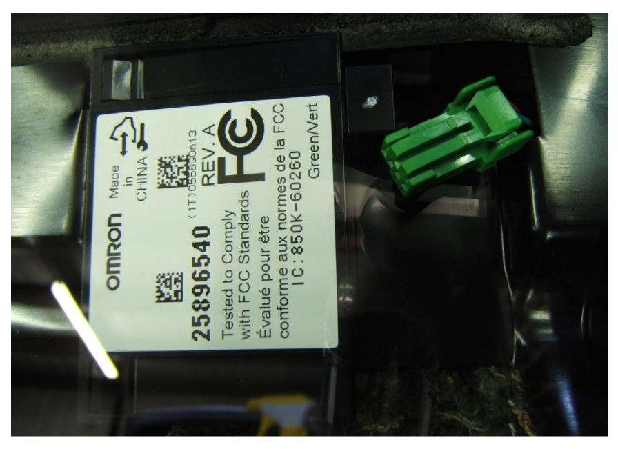
FIGURE 5.20 OMRON TPMS RECEIVER DISCONNECTED FOR MALFUNCTION DETECTION TEST
