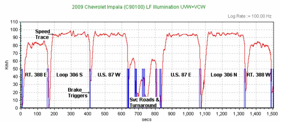
LF Detection Phase: Telltale illumination in 45.5 seconds. Driving above 50 km/h (31 mph) was not required.
