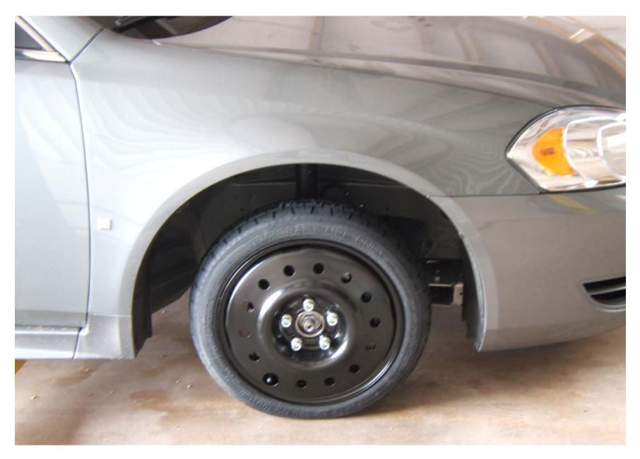
FIGURE 5.19 SPARE INSTALLED ON RIGHT FRONT FOR MALFUNCTION DETECTION TEST
