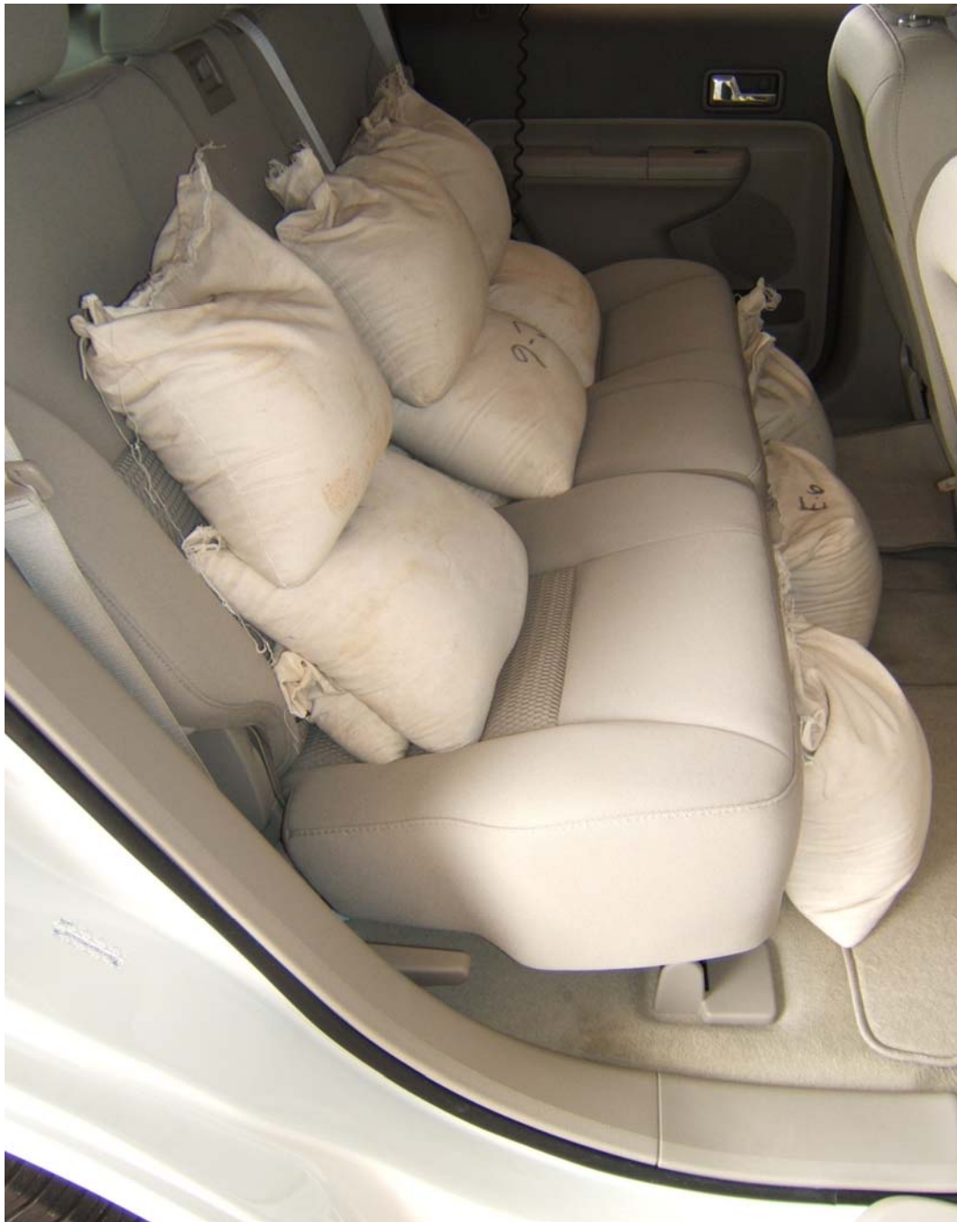
FIGURE 5.14 VEHICLE REAR SEAT BALLAST FOR UVW + VCW LOAD
