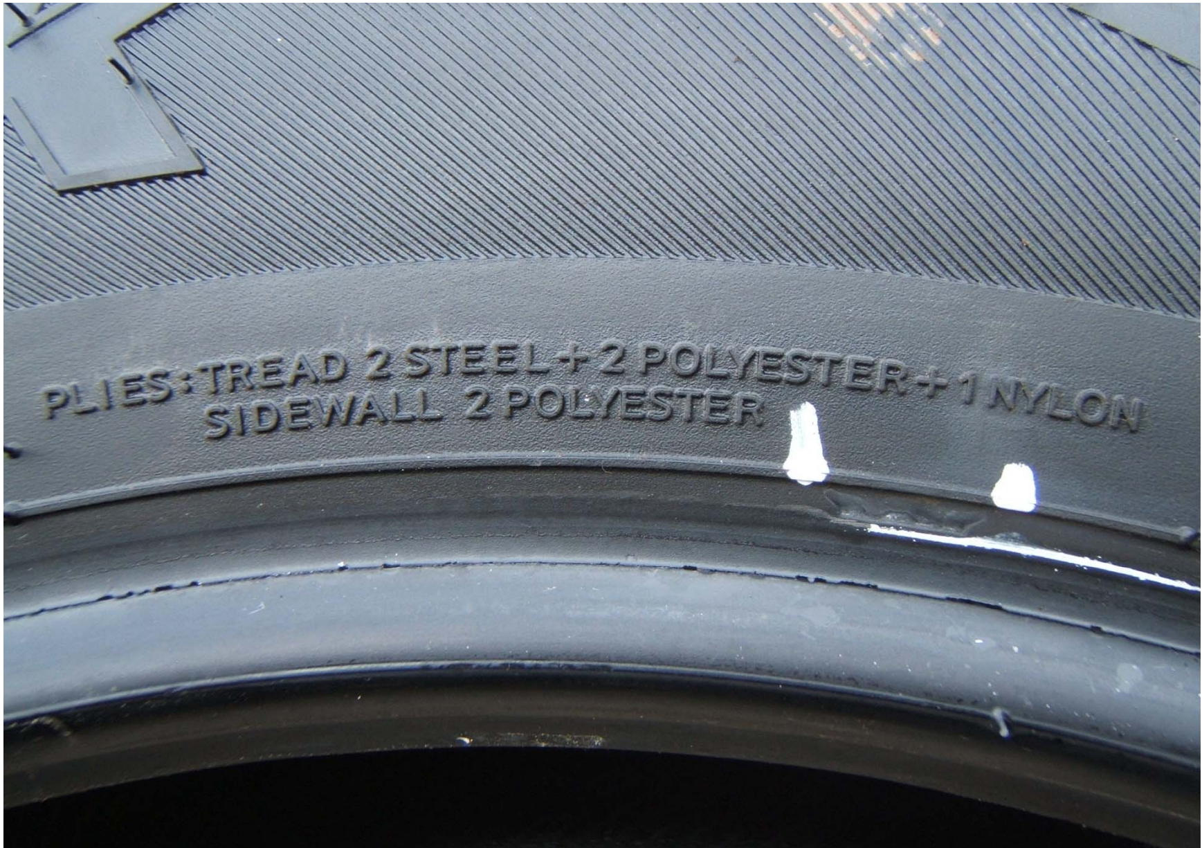
FIGURE 5.9 TIRE SHOWING SIDEWALL / TREAD CONSTRUCTION
