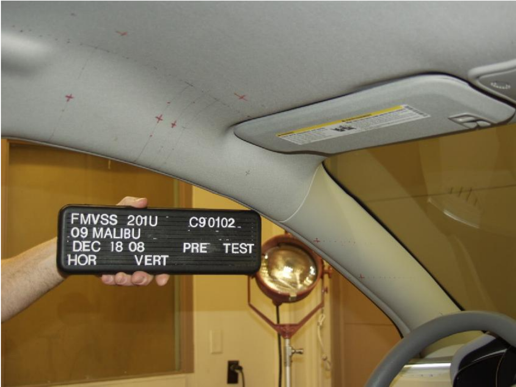
Figure A-7 : PRE-TEST DRIVER SIDE A-PILLAR
