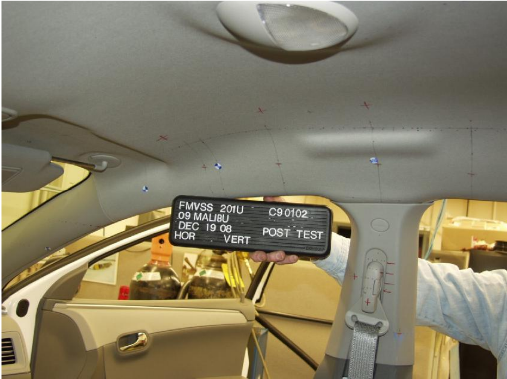
Figure A-24 : POST-TEST PASSENGER SIDE SIDE RAIL
