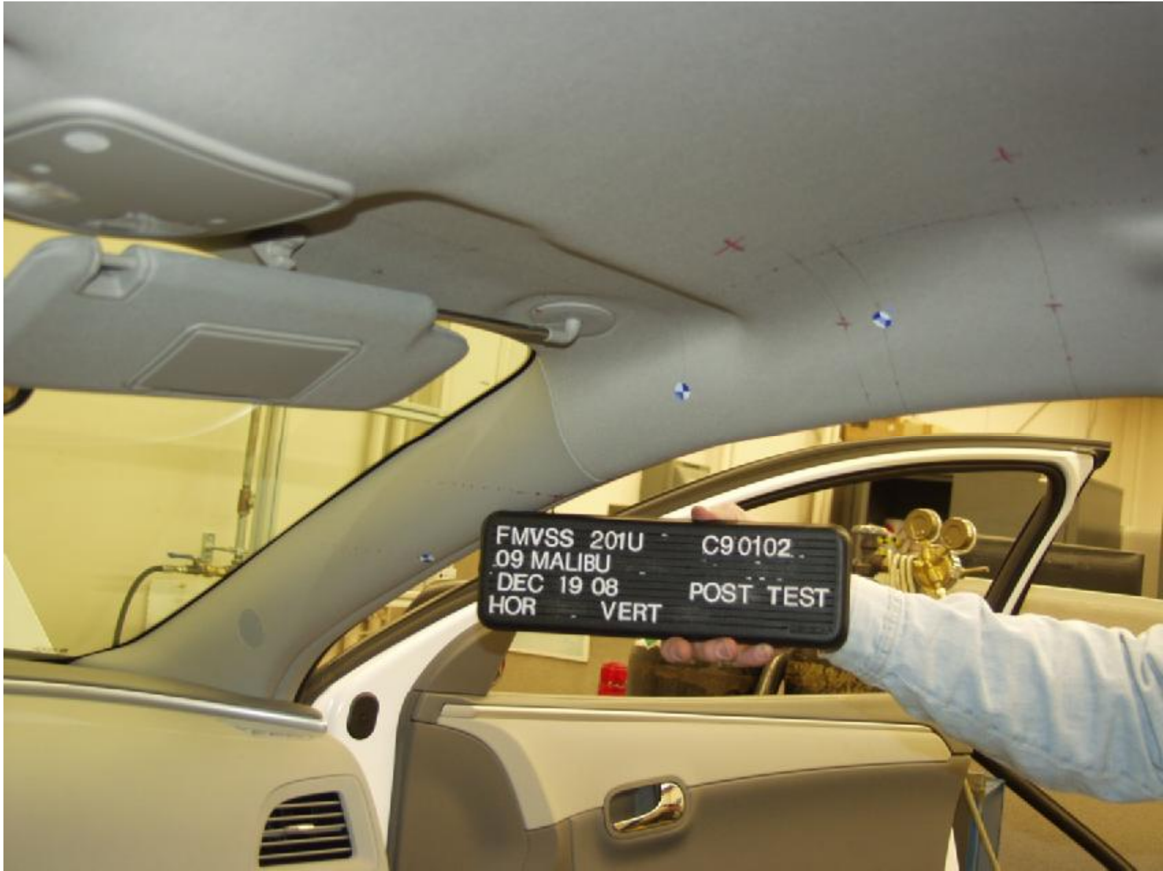
Figure A-22 : POST-TEST PASSENGER SIDE A-PILLAR
