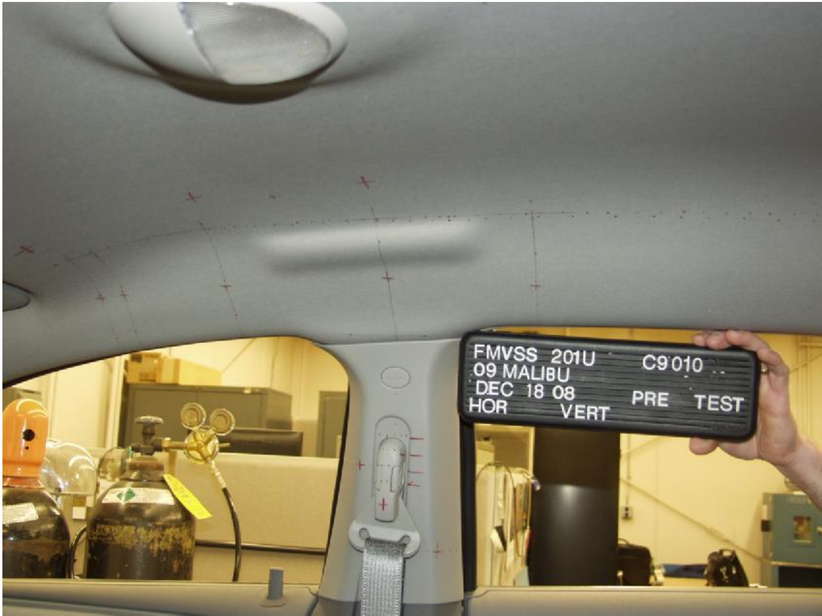
Figure A-15 : PRE-TEST PASSENGER SIDE B-PILLAR
