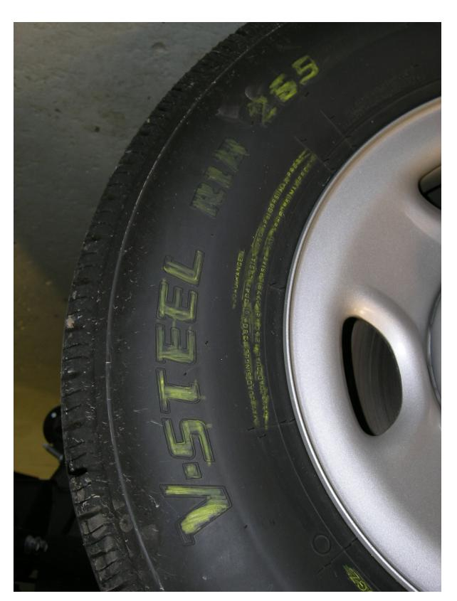
Right Front Tire DOT Serial Number, Tire Load Range Identification and Tire Size Designation
