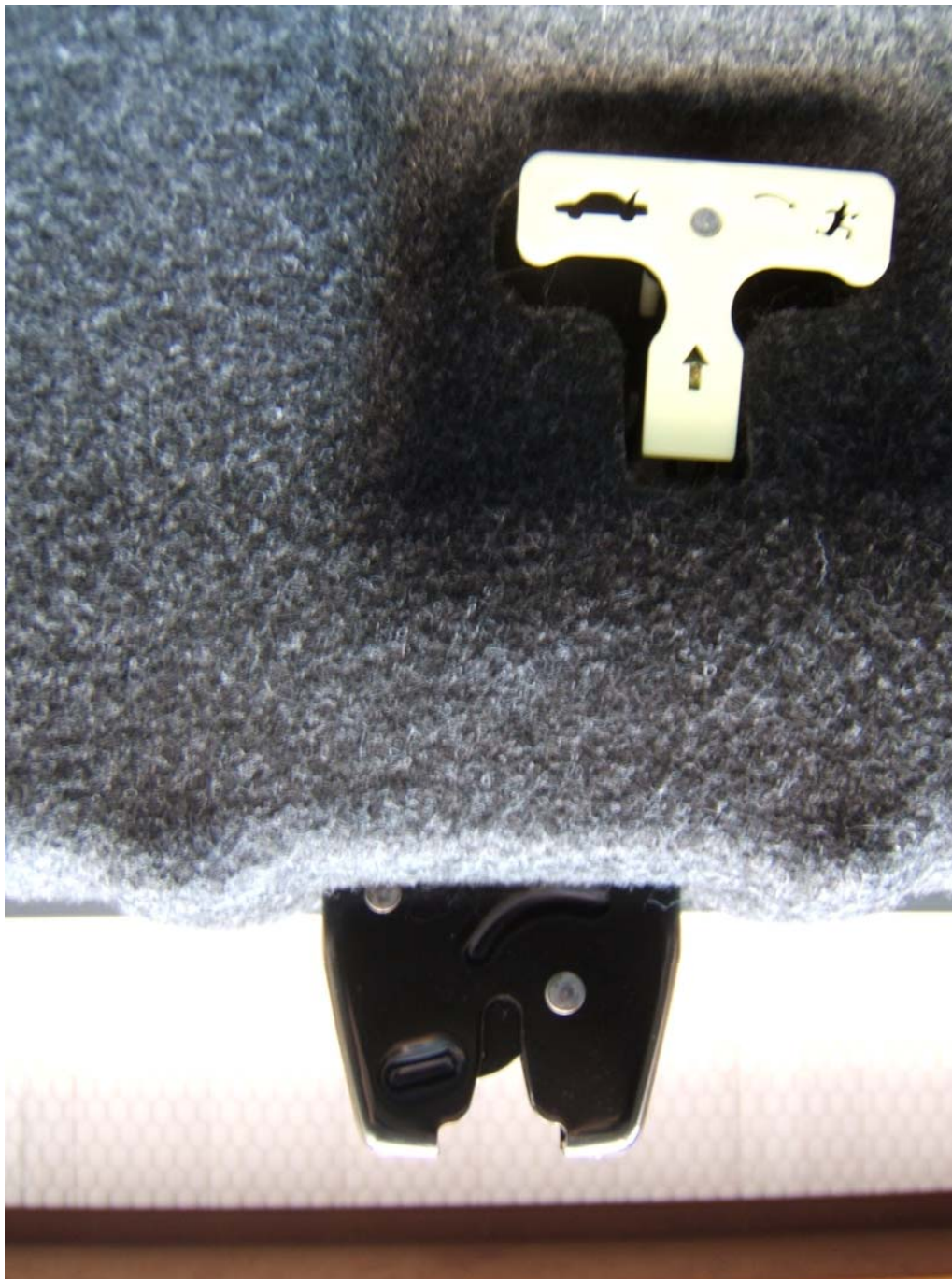
FIGURE 5.8 VEHICLE TRUNK COMPARTMENT MANUAL RELEASE MECHANISM
