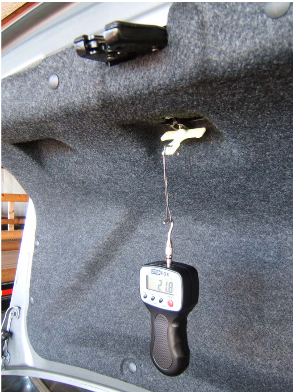
FIGURE 5.9 RELEASE MECHANISM WITH TEST EQUIPMENT ATTACHED
