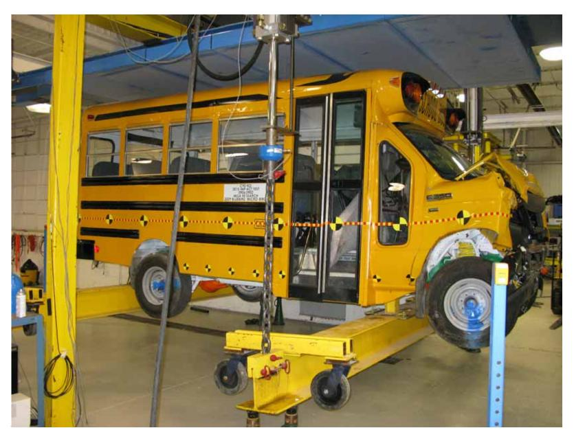
Loading Device Placed Against Bus's Roof at Beginning of Test (Right Front)
