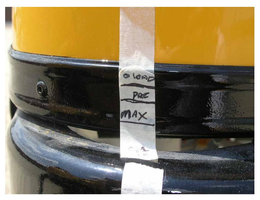
Backup Roof Deflection Measuring Device at Maximum Load Condition (Left Rear)
