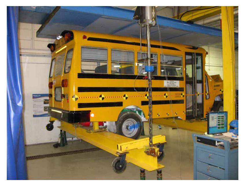
Loading Device Placed Against Bus's Roof at Beginning of Test (Right Rear)
