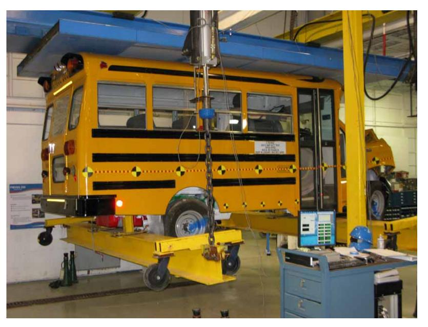
Loading Device Placed Against Bus's Roof at Maximum Load Condition (Right Rear)
