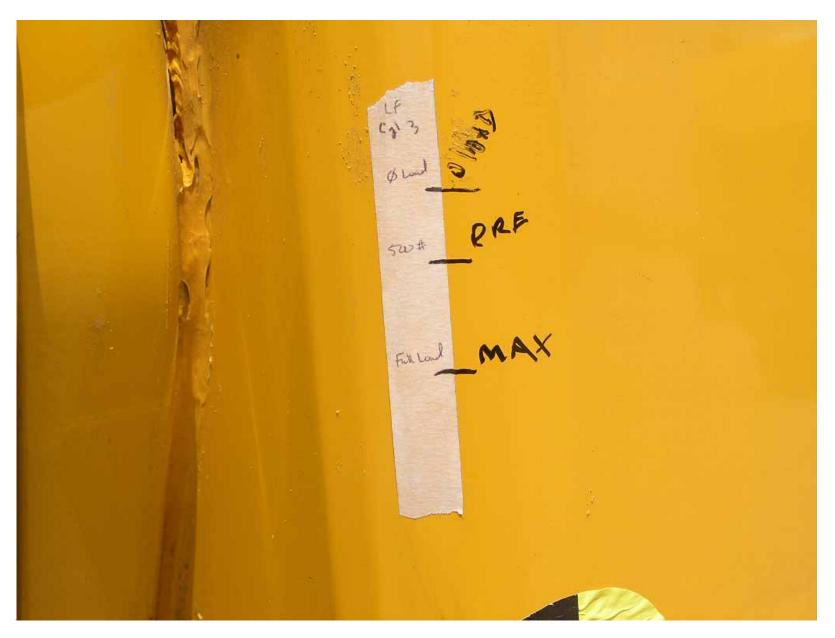
Backup Roof Deflection Measuring Device at Maximum Load Condition (Left Front)
