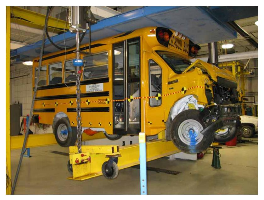
Loading Device Placed Against Bus's Roof at Maximum Load Condition (Right Front)
