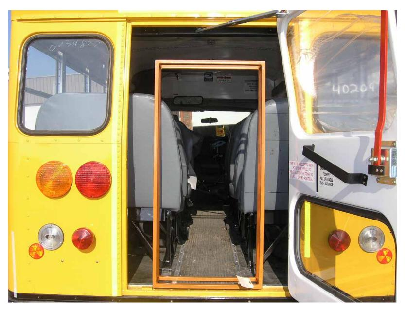
Rear Exit Door Open With Parallelepiped In Place
