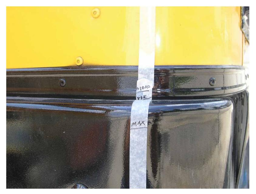
Backup Roof Deflection Measuring Device at Maximum Load Condition (Right Rear)
