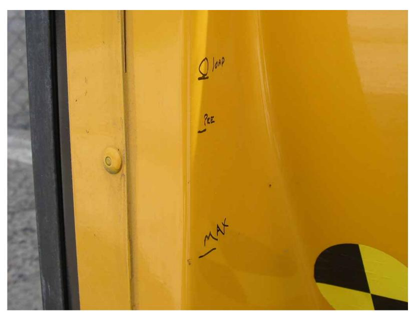
Backup Roof Deflection Measuring Device at Maximum Load Condition (Right Front)
