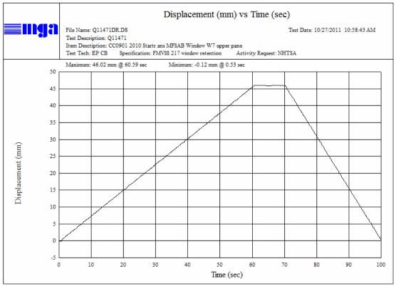
W7 Rearmost Driver Side Upper Window Pane Displacement vs. Time
