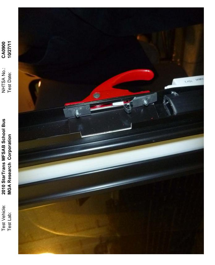
Window Retention Test of W6 Rearmost Passenger Side Lower Window Pane Post-Test Damage
