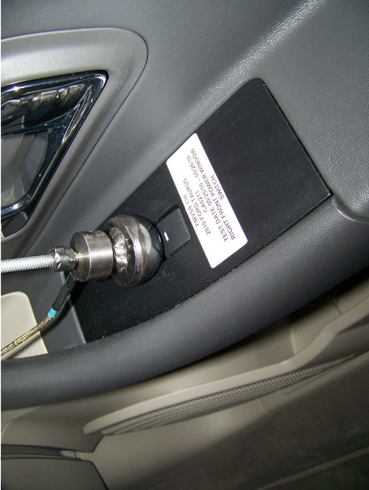
Figure 18: Sphere Test Right Front Window Switch
