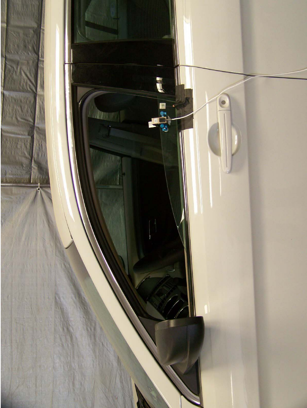
Figure 16: Left Front Window Test Set-Up Rear Edge
