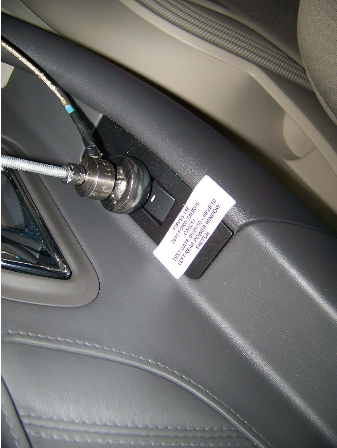
Figure 19: Sphere Test Left Rear Window Switch
