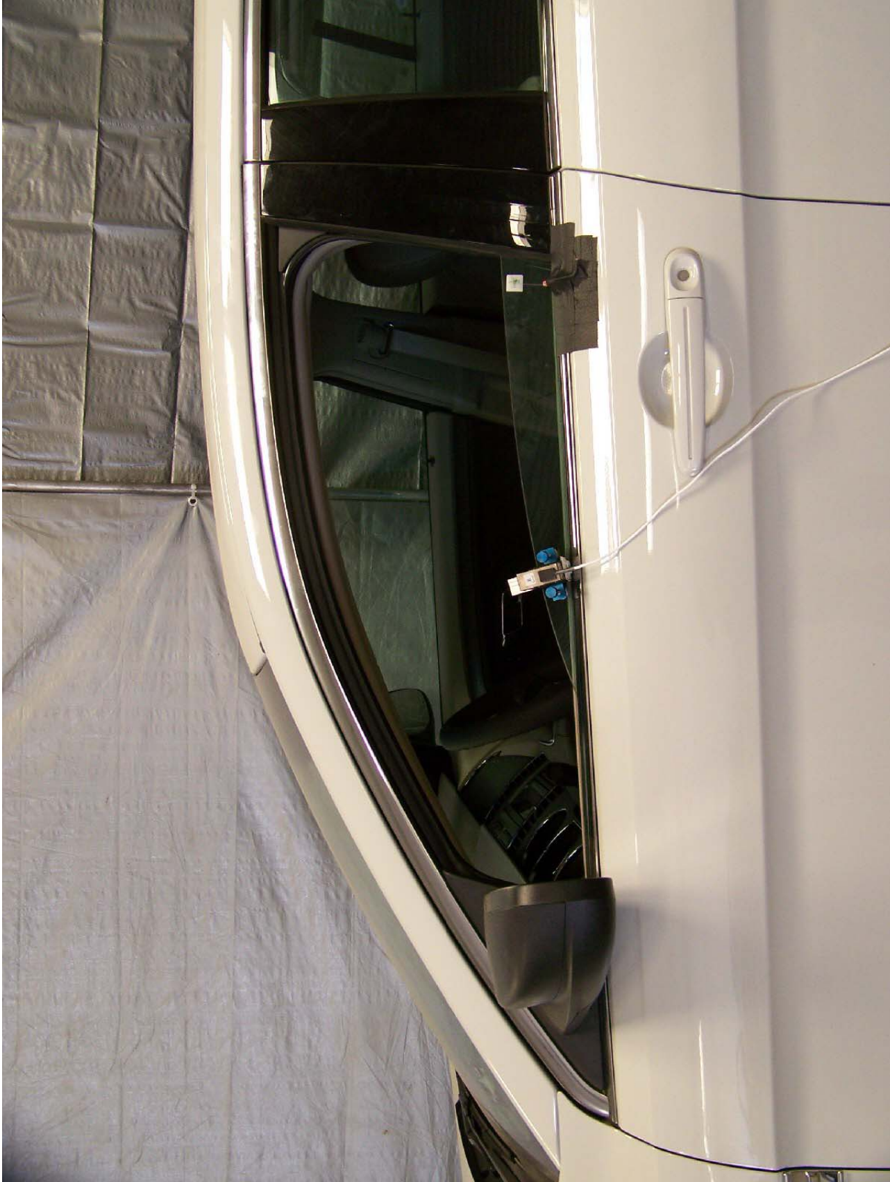
Figure 15: Left Front Window Test Set-Up Leading Edge
