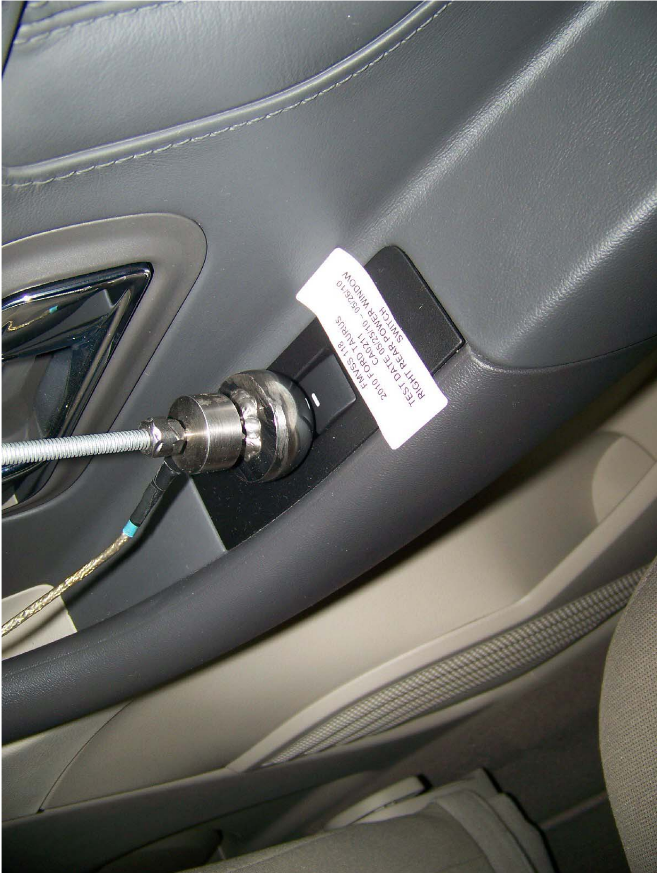
Figure 20: Sphere Test Right Rear Window Switch
