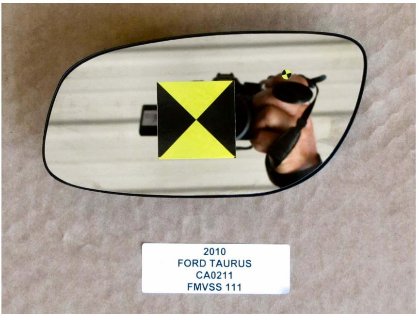
FIGURE 15: MIRROR SET-UP FOR AREA MEASUREMENT
