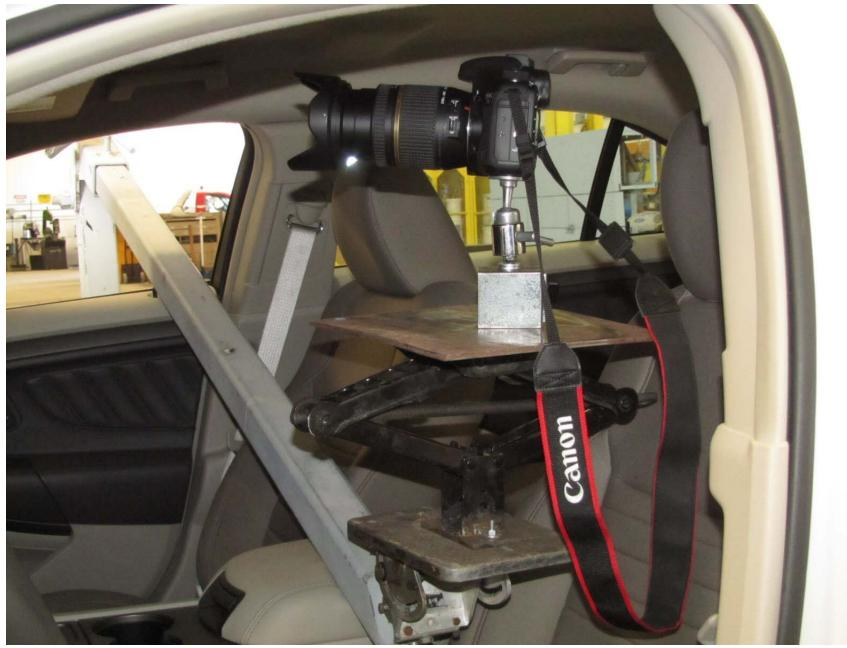
FIGURE 11:CAMERA SET-UP FOR PHOTOGRAPHING REFERENCE BOARD
