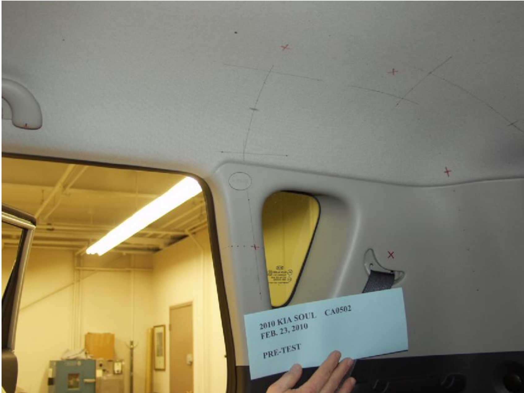
Figure A-19 : PRE-TEST PASSENGER SIDE OTHER PILLAR
