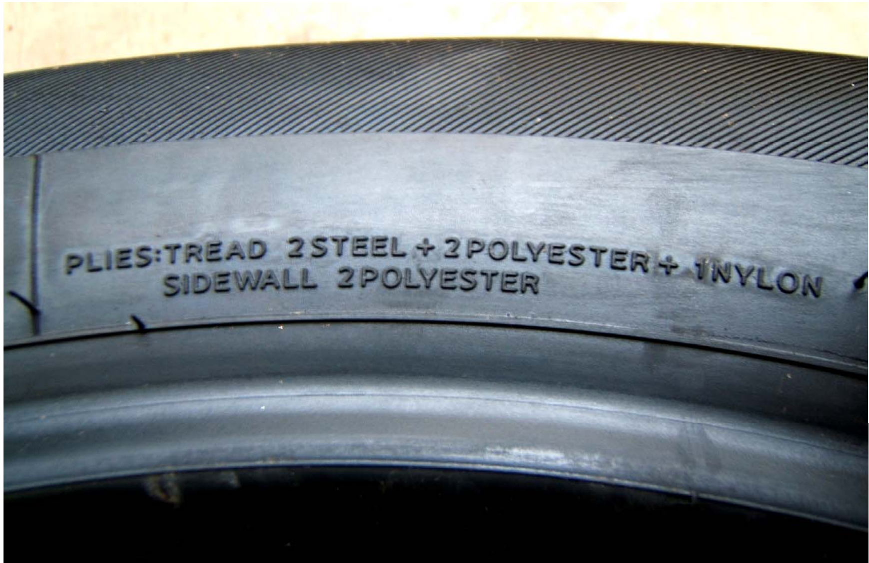
FIGURE 5.9 TIRE SHOWING SIDEWALL / TREAD CONSTRUCTION
