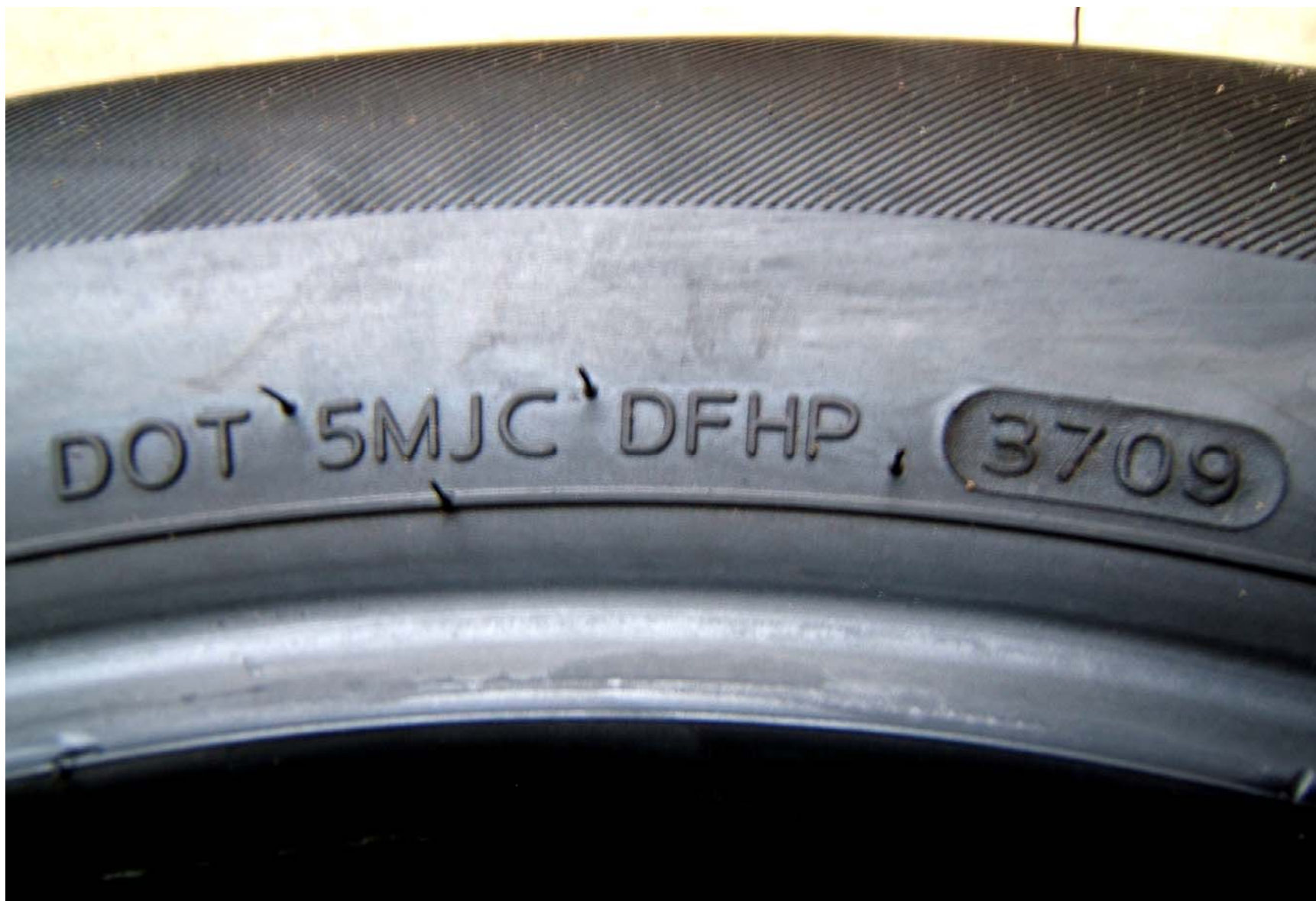
FIGURE 5.7 TIRE SHOWING DOT SERIAL NUMBER
