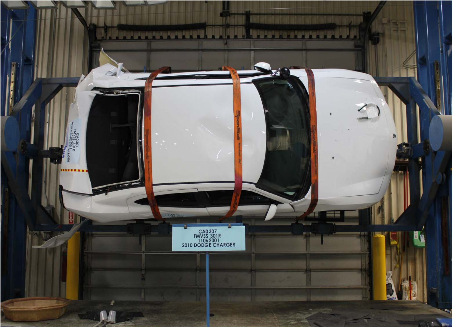
Static Rollover at 270 Degrees
