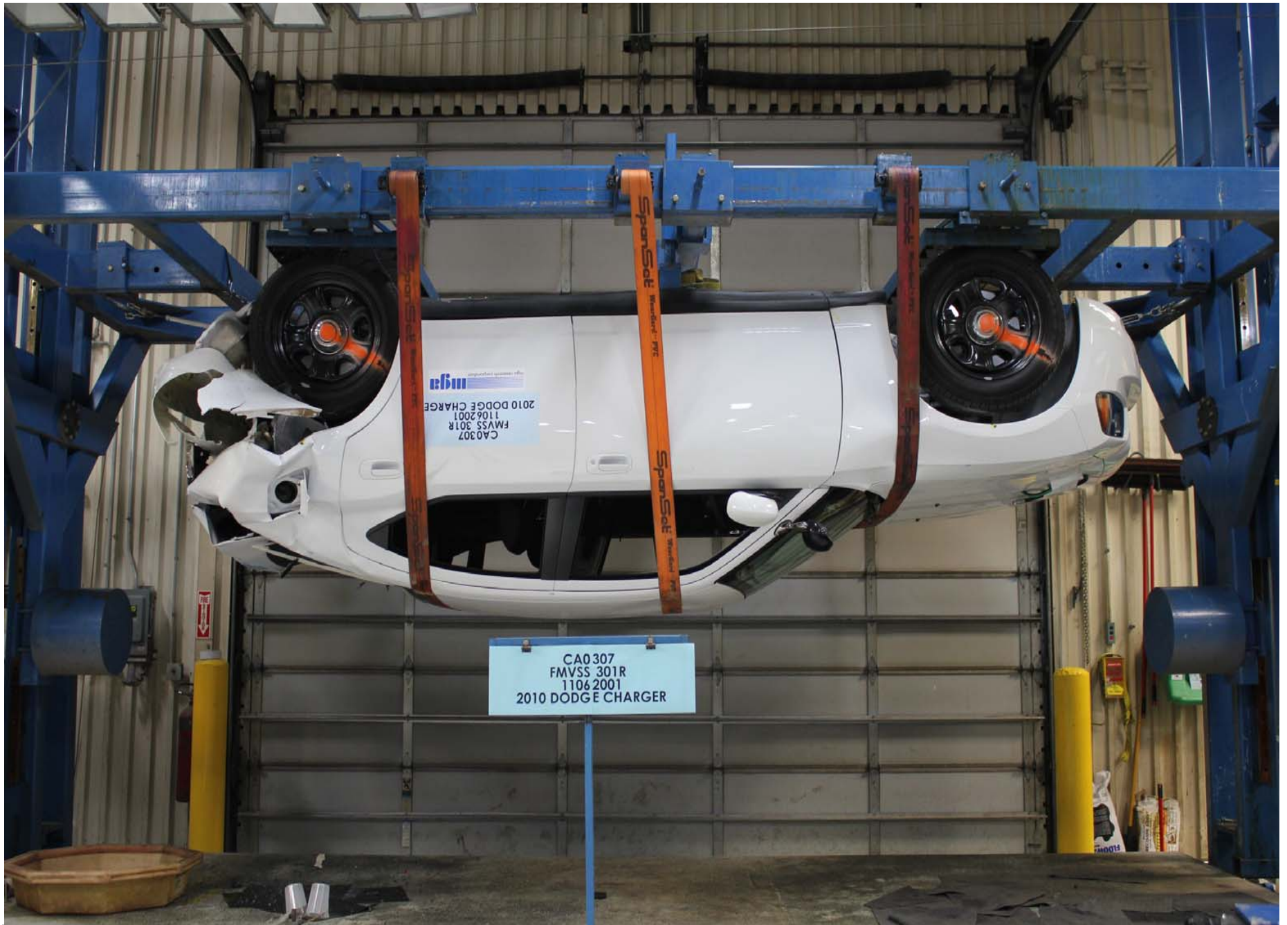
Static Rollover at 180 Degrees
