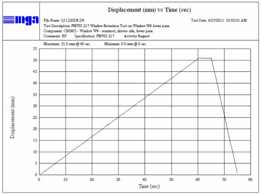
W4 Rearmost Driver Side Lower Window Displacement vs. Time
