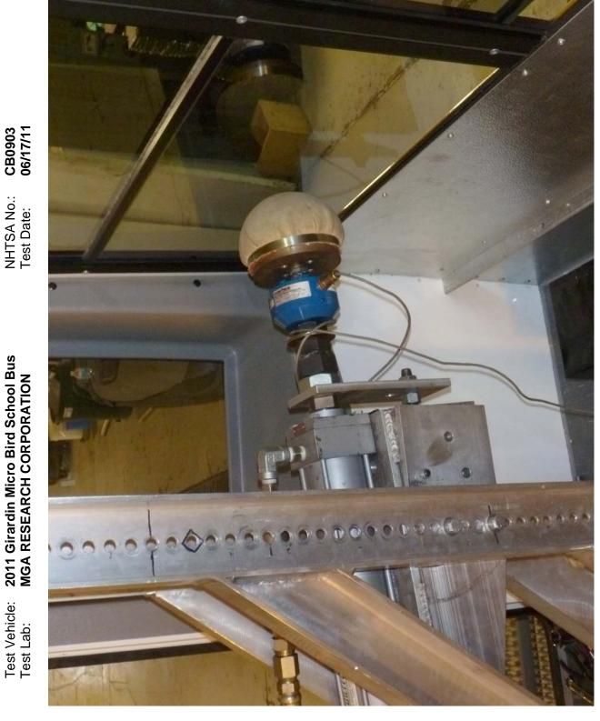
Window Retention Test of W4 Rearmost Driver Side Lower Window (Post-Test)
