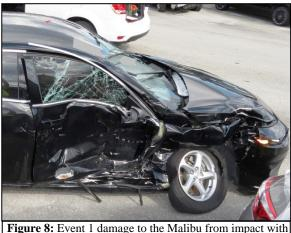
**Figure 8:** Event 1 damage to the Malibu from impact with the Tahoe's front plane.
