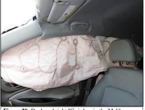
Figure 20: Deployed right IC air bag in the Malibu.
