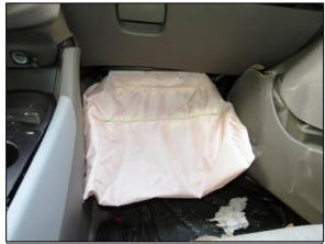
Figure 17: Deployed front right passenger's knee air bag in the Malibu.
