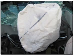
Figure 16: Deployed passenger's frontal air bag in the Malibu.
