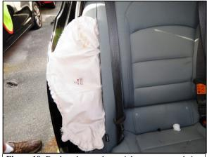
Figure 19: Deployed second row right seat-mounted air bag in the Malibu.
