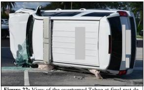
**Figure 22:** View of the overturned Tahoe at final rest depicting undamaged planes (on-scene image obtained from the investigating law enforcement agency).
