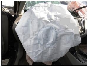
Figure 14: Deployed driver's frontal air bag in the Malibu.
