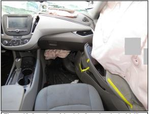
**Figure 10:** Intrusion of the right front door in the Malibu as viewed from above the front row right seat position.
