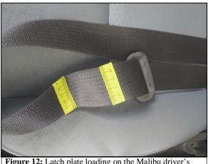
Figure 12: Latch plate loading on the Malibu driver's seat belt webbing.
