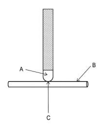
A – Edge Sensor B – 1-7/8" Diameter Cylinder C – 15 Pound Force
