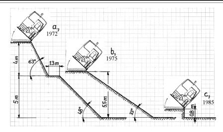
**Figure 3:** Three different rollover tests Hungary<sup>70</sup> evaluated for ECE R.66 development. Test conditions "a" and "b" produce an initial contact between the bus and ground that may distribute the crash load into more of the bus sidewall structure than test condition "c." Test condition "c" concentrates the initial rollover impact load into the upper outer corner of the bus superstructure.
