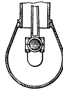
CRANK IN DEAD CENTRE POSITION.
