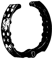
CORK INSERTS USED IN AUTOMOBILE BRAKE.
