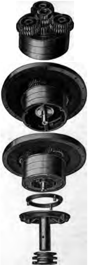
Figure 52.—Transmission and Clutch Partly Assembled
