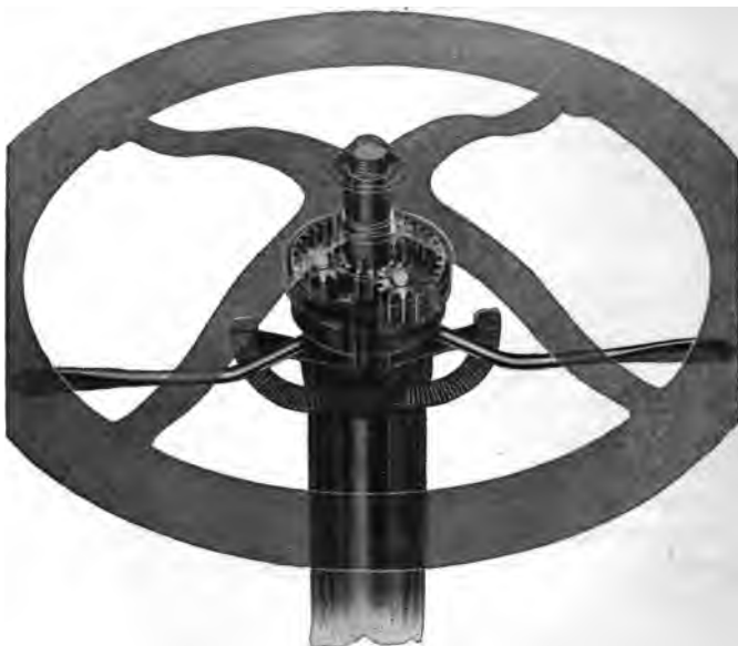
Figure 33.—Steering Wheel and Gearing.
