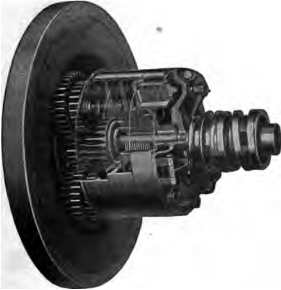
Figure 21.—The Transmission and High Speed Clutch.
