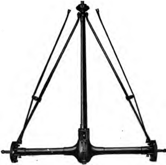
Figure 26.—The Rear Axle and Drive Shaft Assembly.
