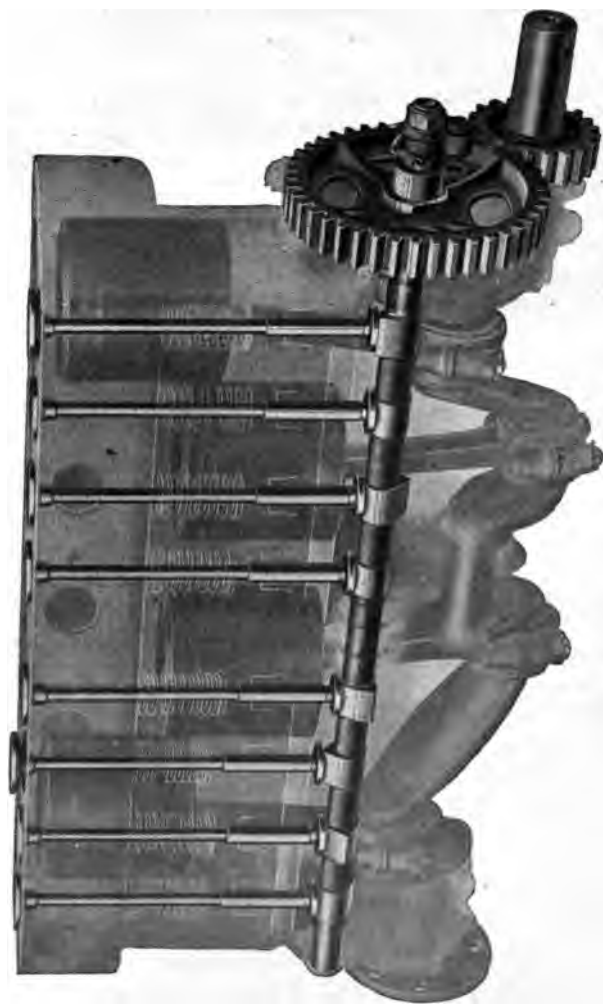
Figure 4.—Valve Operating Parts of the Ford Engine.
