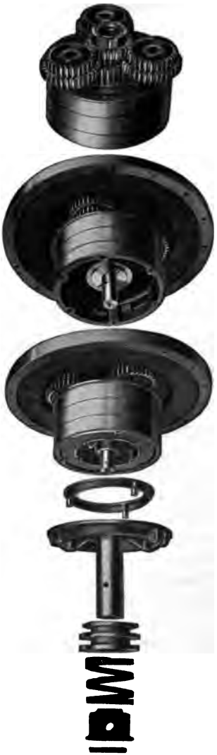
Figure 52.—Transmission and Clutch Partly Assembled
